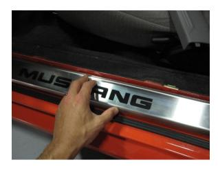
**Step 5:** Replace the factory plastic inner trim to complete the installation.
