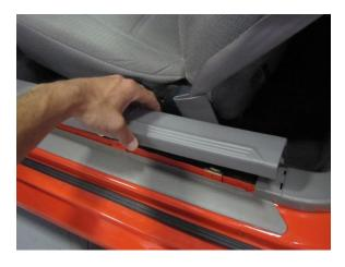
**Step 2:** Remove the outer plastic factory trim by prying gently with a plastic scraper or similar.
