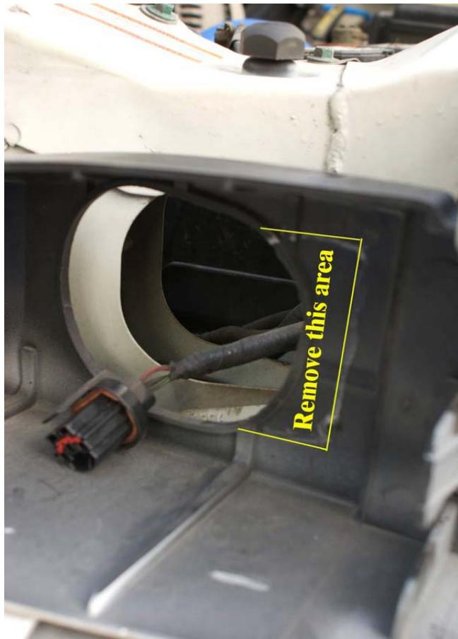
8. Using a Dremel tool with plastic cutting tip, or similar tool, remove the plastic in the area shown. Make sure you wear safety glasses! Be careful not to cut into the wires behind the plastic.
