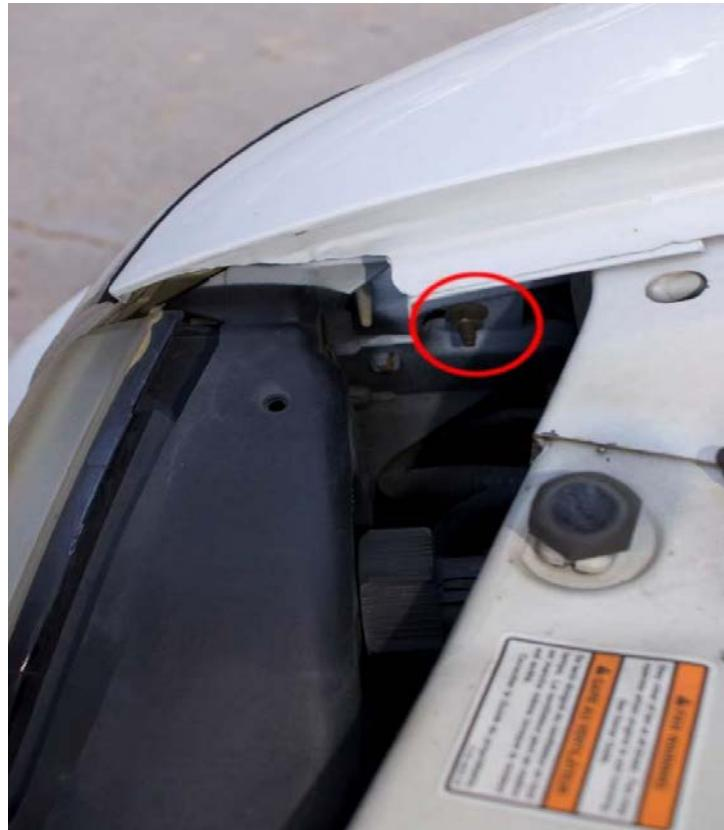
2. Rotate the headlight bulb retaining collar counter-clockwise to release it. Pull out the bulb and unplug from the connector.
