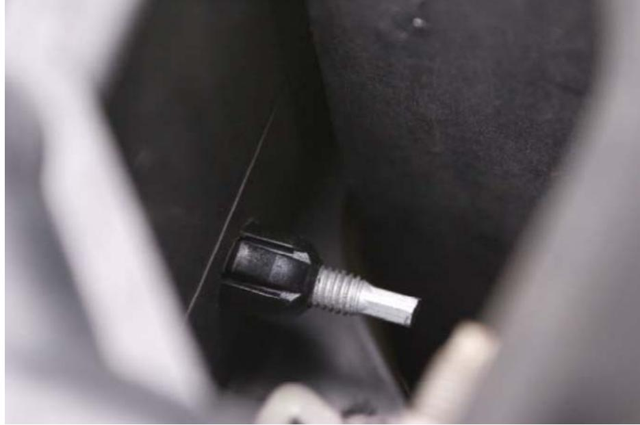
6. The third, the one on the top nearest the fender of the car, will need to have the "L" shaped bracket replaced to hold it in place. This may require the use of pliers or other strong tool if you can't replace with your fingers. The adjustor is shown below prior to installing the "L" shaped bracket.
