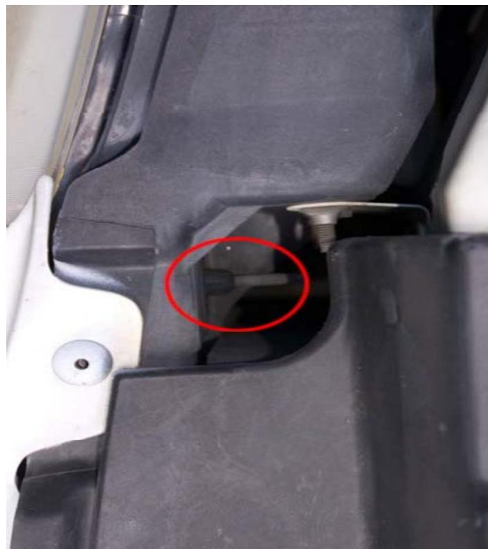
4. On the lower adjustment bolt, there is a plastic retaining device that has two small “ears” on it. One on top and one on bottom. Take a flat-blade screw driver or your fingers and depress the top ear and bottom ear if you can. Pull the headlight assembly out. It may take a little work to get both ears depressed and the headlight removed. Be patient.
