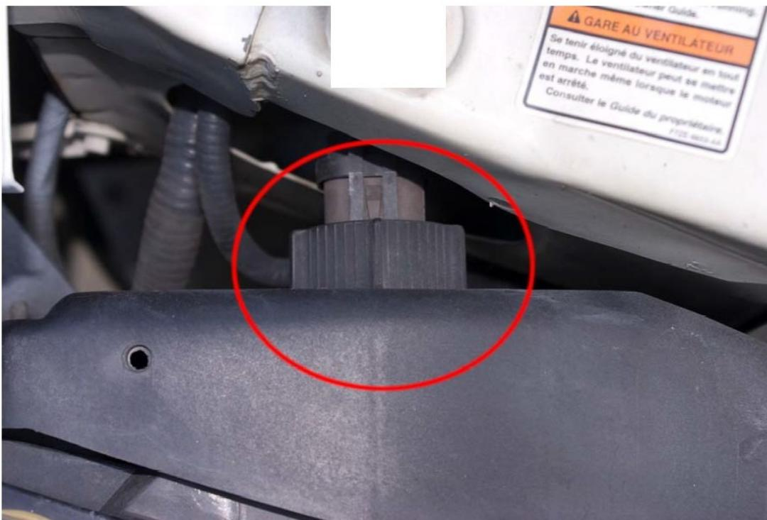
3. Next, take your fingers or a pair of needle-nosed pliers and remove the "L" shaped clip that holds the upper adjustment screw. Pull up on the clip to remove.
