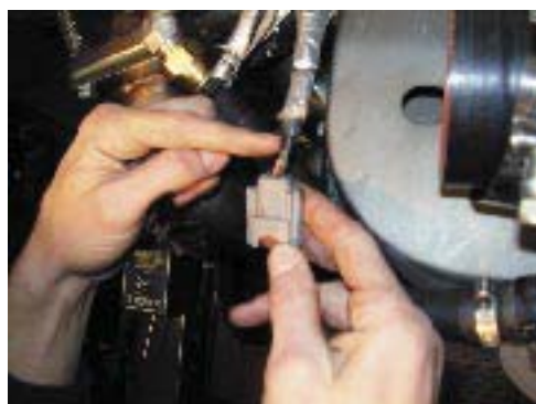
116. Ground oil pump and relay to ground on driver's side radiator core support (refer to wiring diagram for assistance with wiring the pump.)
