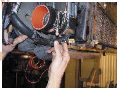
114. Install pump into hose clamps and tighten
