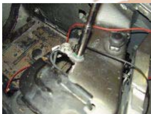
116. Ground oil pump and relay to ground on driver's side radiator core support (refer to wiring diagram for assistance with wiring the pump.)
