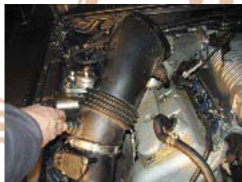
120. Remove factory air inlet assembly, detach mass air meter
