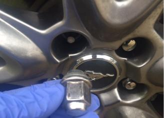
3. Attach key lock to lug nut wrench. Now use this to install new chrome wheel locks.
