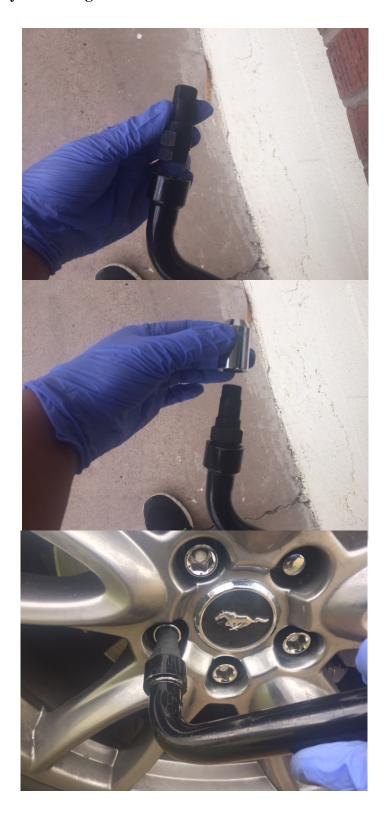
4. When mounting wheel back to vehicle, remember to install wheel locks in an alternating pattern which is also referred to as the star pattern. Simply tighten lugs in the pattern as shown underneath. This helps the wheel fit evenly against mounting surface and also prevents any uneven lug nut torque values. This is crucial to insure that wheel is securely fastened to vehicle.
