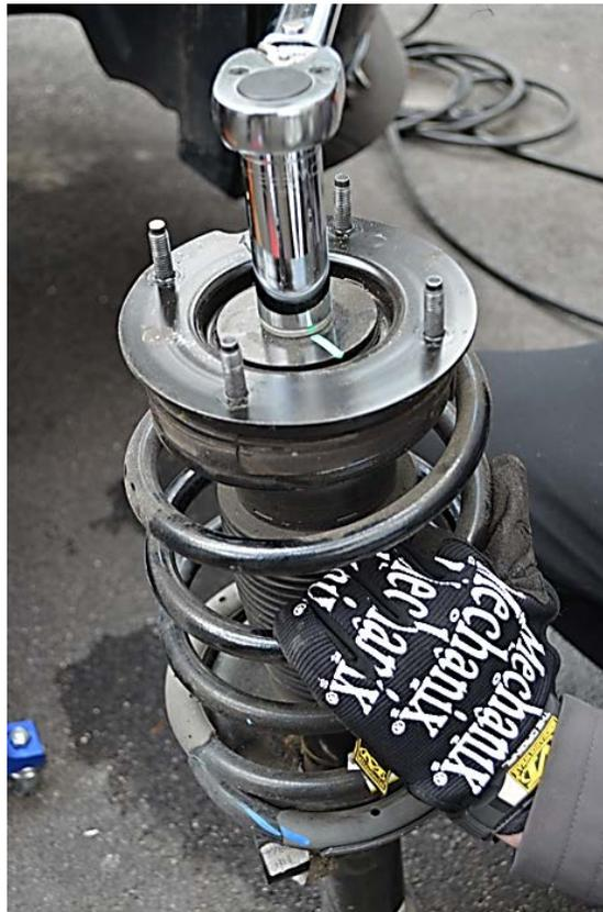
19. Once removed, disassemble the top mount by removing its rubber spring isolator. Use a flathead screwdriver to pry it off gently. You will reuse the rubber spring isolator part of the factory strut mount.
