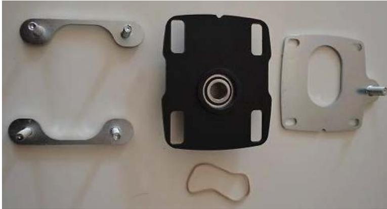
4. Assemble in the following order: Place the camber plate (black) onto the (2) stud plates. Notice that the stud plates have a “U” shape and they point inwards. Also take notice that the camber plate has the bearing protruding on one side only, this side must face down.
