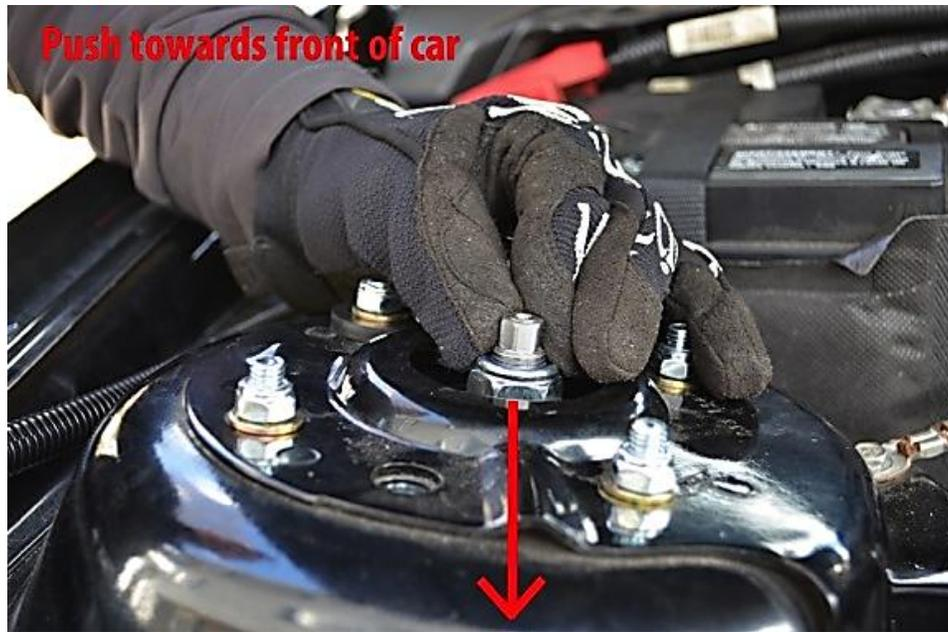
37. Once the strut is pushed all the way forward, tighten the largest support nut using a 17mm socket to 26 ft/lbs. This is the caster adjustment.
