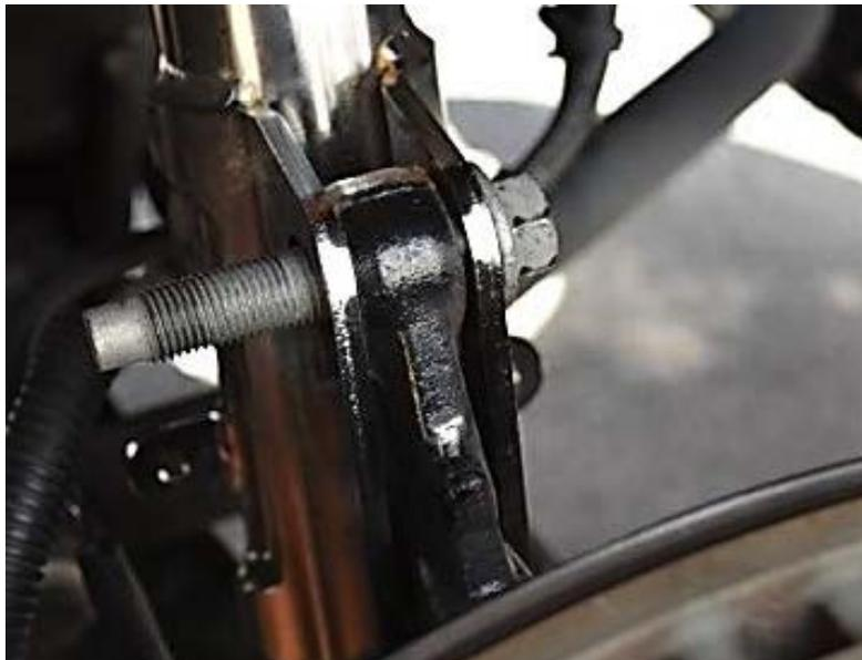
33. Reattach the brake line bracket to the rear of the shock with the 10mm bolt.
