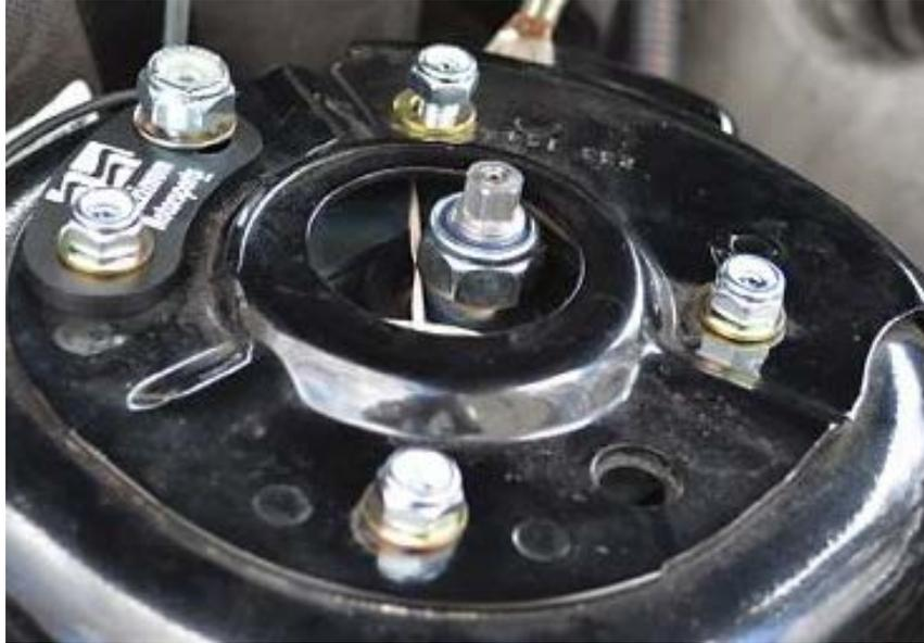
30. Gently tighten all the nuts using the 13mm (small) and 17mm (large) sockets. You do not need a specific torque at this point; simply gently tighten them with a socket wrench. We will come back and loosen them later for adjustment.
