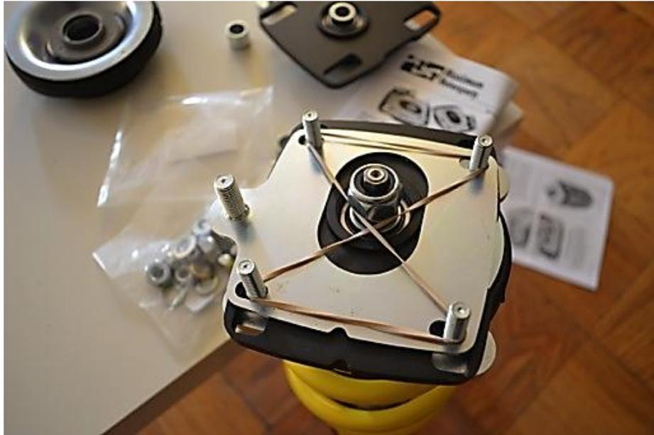
26. Once the top nut is properly tightened, slowly decompress the spring by releasing the tension on the spring compressor. Ensure that everything is lined up as the spring expands. Make sure the rubber spring isolator on the top is lined up with the end of the spring coil. Also make sure that your spring is properly seated into the strut at the bottom.
