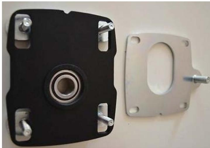
5. Place the caster plate (silver) on top of the camber plate (black) and through the studs. The center oval slot will fit exactly into the center circle of the caster plate. Note that while there is no driver/passenger side differentiation, the (2) notches must match up for correct orientation.
