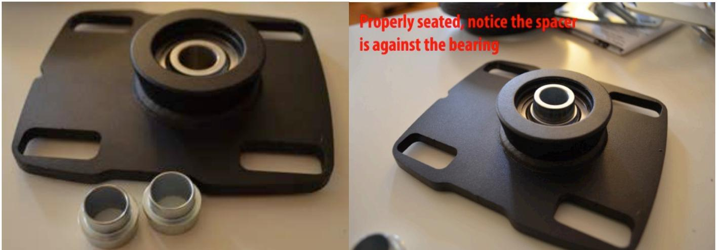
2. Once both sides of the bearing have a taper, do the same for the other caster plate. During the rest of the guide, make sure these don't fall off the plate.
