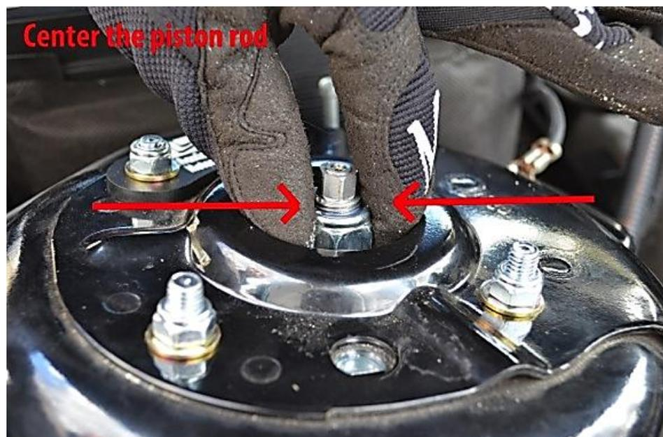
39. Once centered, tighten the remaining (4) nuts using a 13mm socket to 20 ft/lbs.
