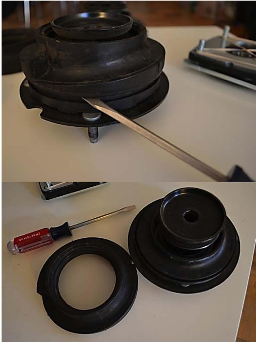
20. With the spring still compressed and the top mount off, locate the rest of the spacers. The following is a picture of the types of spacers you should have, viewed from both angles. Note that we've already used the (4) tapered spacers on the camber plates (the 2 rows on the right of the picture). The remaining spacers have (2) types: (1) long and (1) short.
