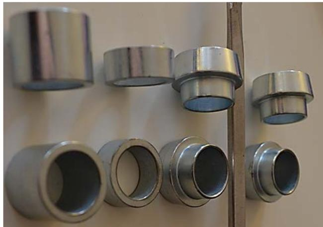
21. Slide the long spacer first so that it is below the short spacer, as shown. **Note:** the pictures show an aftermarket suspension, but the process is exactly the same with factory suspension or just about any bolt-on suspension. The piston rod is 22mm in diameter, which is typical.
