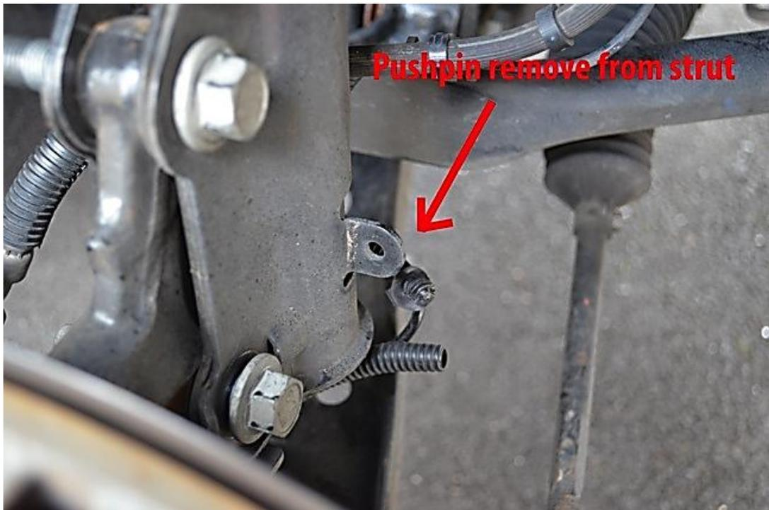
14. Remove sway bar end link by loosening and removing the bolt that holds it to the strut. Use a 15mm deep socket here as a shallow socket will not work.
