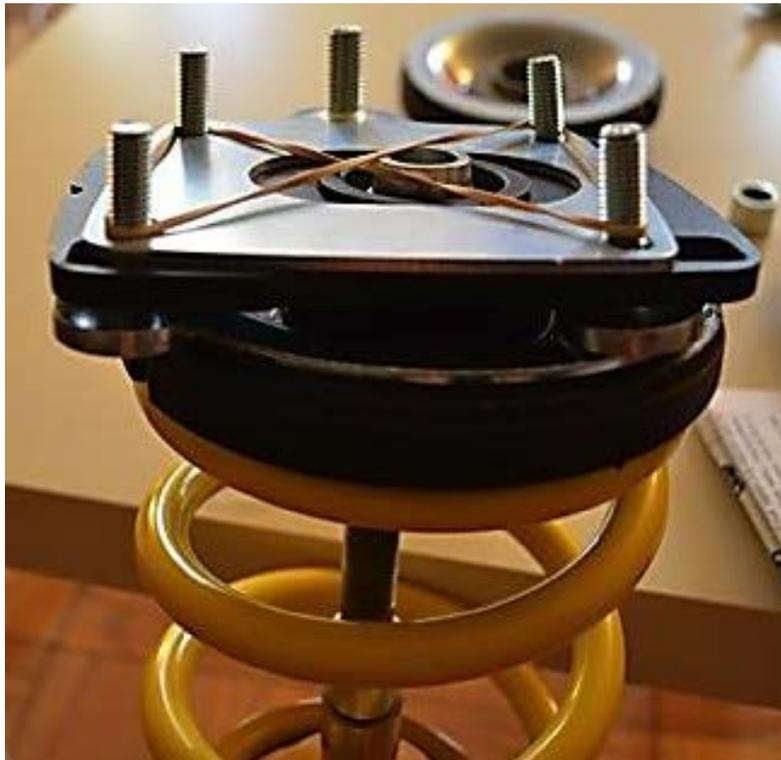
25. Tighten the top strut nut back onto the piston rod using a 21mm socket. **IMPORTANT:** Refer to your shock manufacturer for torque specifications. Each shock manufacturer has different torque recommendations for the top strut mount. OEM spec is 45 ft/lbs. You may need to clamp the piston rod if it rotates. Be sure not to damage the piston rod during this process; vice grips with towels for padding works well.
