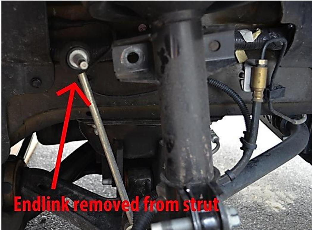
15. Use your floor jack to support the hub assembly. When you remove the strut, the hub will be unsupported and would otherwise fall to the ground. To avoid this, gently support the hub by the brake rotor. You can also support the suspension arm if you prefer.
