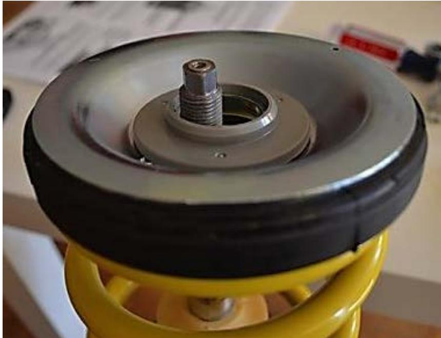
24. Now place your assembled camber caster plates on top of the metal dish. Note that the protruding spherical bearing faces down and the studs face up. The bottom of the camber plate (black) will fit perfectly around the plastic ring shown in the previous picture. Make sure that both tapered spacers are still seated in the spherical bearing when you put the plates on. The piston rod will fit through the tapered spacers and through the spherical bearing.
