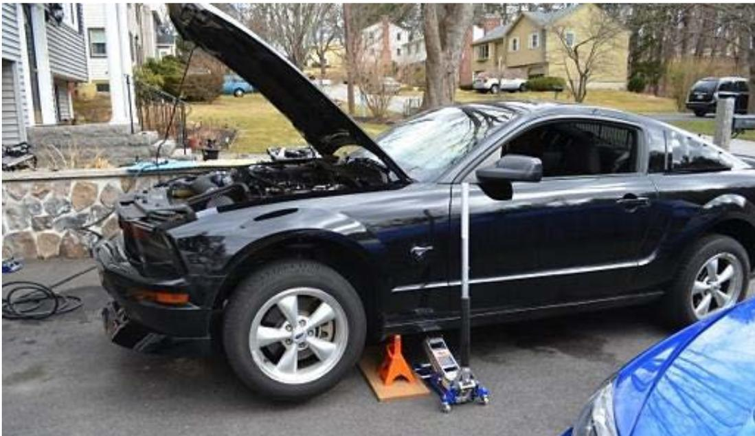
10. Remove both front wheels to reveal the strut assembly. The strut assembly is attached by (2) bolts and nuts on the wheel hub. It is attached to the chassis with (4) nuts at the strut tower (under the hood). But before we remove the strut, we need to remove the ABS line, brake bracket, and the swaybar end link, which are all attached to the strut.
