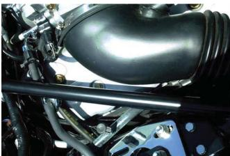
Be sure that both firewall mounts of the brace are held down against the firewall pinchweld.
