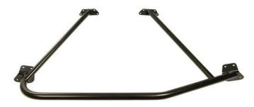
The MM Strut Tower Brace attaches to each strut tower and to the firewall.
