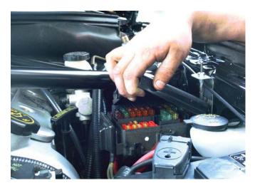
NOTE: If the fuse box cover cannot be opened, reposition the fuse box by moving it forward. This can easily be done by slipping a screwdriver between the front of the strut tower and the rear of the metal fuse box mounting tabs (these are attached to the strut tower). Gently pry the tabs forward. This will move the fuse box slightly forward.
