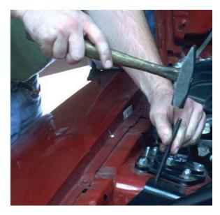
13. Center punch the mark. Drill a 1/8" pilot hole. Drill out to 5/16". Deburr the hole.
