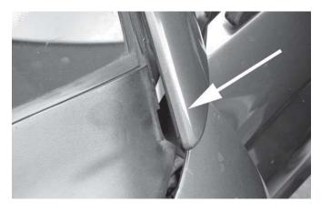
19. Remove the plastic cowl cover at the base of the windshield. It is held on with clips. Remove it by gently prying it upwards. When it is loose, disconnect the hose to the windshield washer nozzles (pointed to below).
