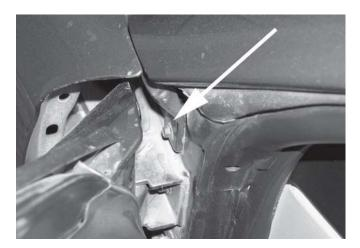
18. DO NOT remove the applique. Gently move it away just enough to open a small gap for removal of the plastic cowl at the base of the windshield.
