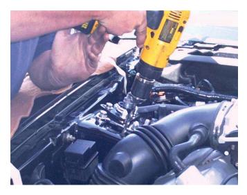
14. Set the Strut Tower Brace back into place. Insert a 5/16" bolt into the hole to hold the brace in position. Hold it both downwards and rearwards. Mark the positions of all of the other holes on both strut towers. Unclip the relay box from the inner fender panel to provide access for marking and drilling the hole. Remove the Strut Tower Brace before drilling.
