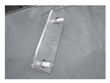
25. Line up the nutplate on the 5/16" holes drilled in the firewall in Step 19. Use the bolts installed in the previous step as guide pins. Make sure that the small hole in the plate is biased downward.
