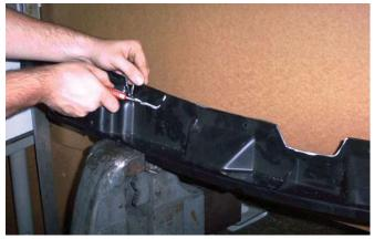
Put the plastic back into position on the firewall.
