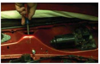
33. Install the #8 sheet metal screw into the small hole in the nutplate. Remove the 5/16-18 bolts.
