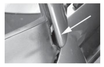
19. Remove the plastic cowl cover at the base of the windshield. It is held on with clips. Remove it by gently prying it upwards. When it is loose, disconnect the hose to the windshield washer nozzles (pointed to below).
