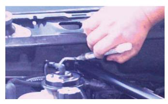
7. Remove the Strut Tower Brace.
