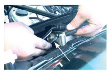
20. Place the Strut Tower Brace back into position. Place flat washers under the heads of (6) 5/16" x 1" long bolts. Place the bolts through each of the holes at the strut towers. This is for positioning only. Do not install the nuts. 21. Hold the brace down and rearwards. Mark the position of the 8 holes at the firewall.
