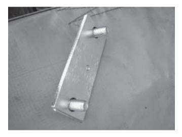
25. Line up the nutplate on the 5/16" holes drilled in the firewall in Step 19. Use the bolts installed in the previous step as guide pins. Make sure that the small hole in the plate is biased downward.
