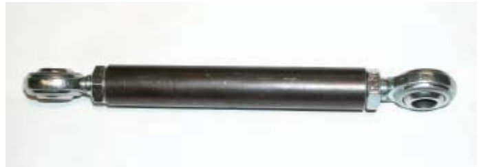
Incorrect- The rod ends are not aligned
