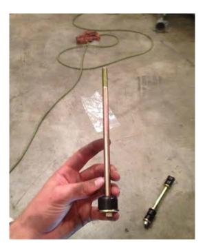
Step 2: Feed the new end link up through the hole from under the control arm.
