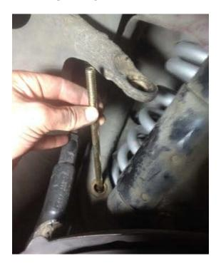
Step 3: Next slide another bushing on the new end link bolt followed by a washer, the spacer sleeve, another washer, and another bushing.
