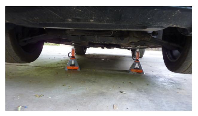
3) Raise the front end of the car, on a solid flat surface, so there is enough room for you to work freely. Make sure to keep the car lifted up with the use of jack stands and NOT the jack/lift alone. Make sure the E-Brake is on to prevent rolling of the vehicle.
