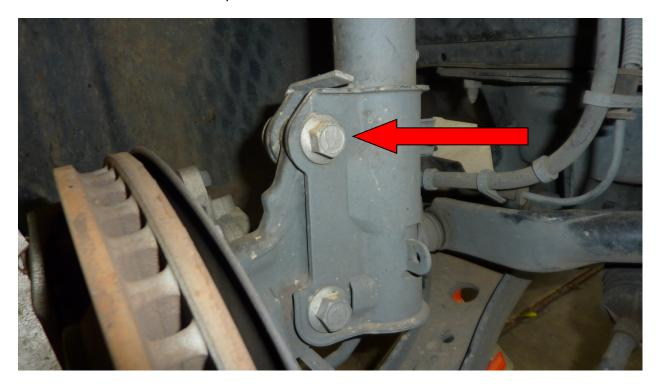
6) Use your 18mm socket to loosen the top strut bolt. You will see that the bolt will turn and so will its clip from the other side of the spindle. This will spin until it binds up with the rest of the spindle. It will then loosen as you spin the bolt.
