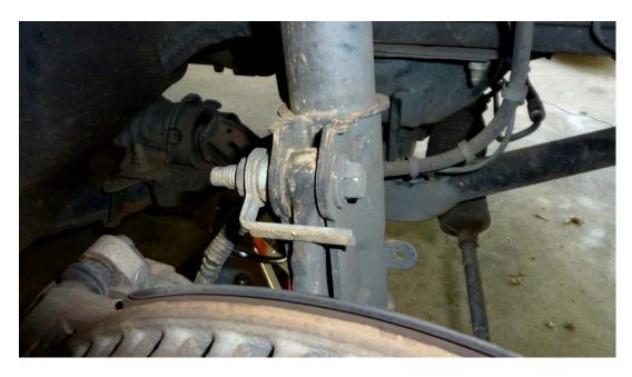
7) Remove the top strut bolt and prepare to install the camber adjustment bolt.
