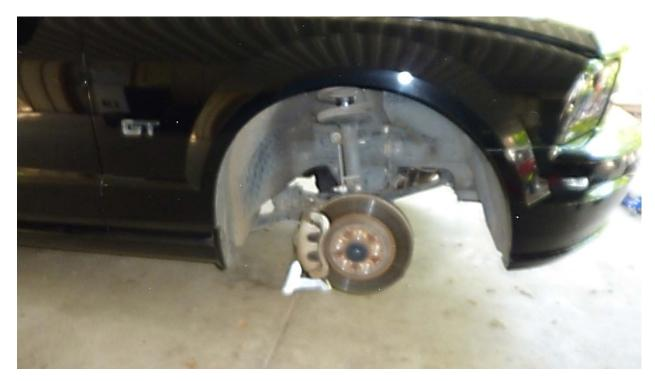
5) The camber bolt is easy to locate and can be located behind the brake disks on the spindle. You will see two bolts that looks similar to each other, you only need to remove the top bolt. The strut bolt that needs to be removed is indicated by the RED arrow below.
