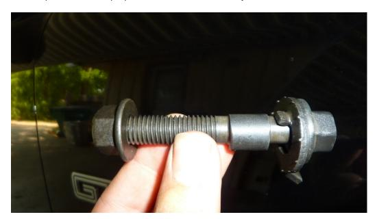
8) You will see the end of bolt that has a lobe on it, this is the end of the bolt the will face to the front bumper once installed. The "toothed" washer will rest on the outside of the spindle. Once installed correctly, your set up should look like the picture below.
