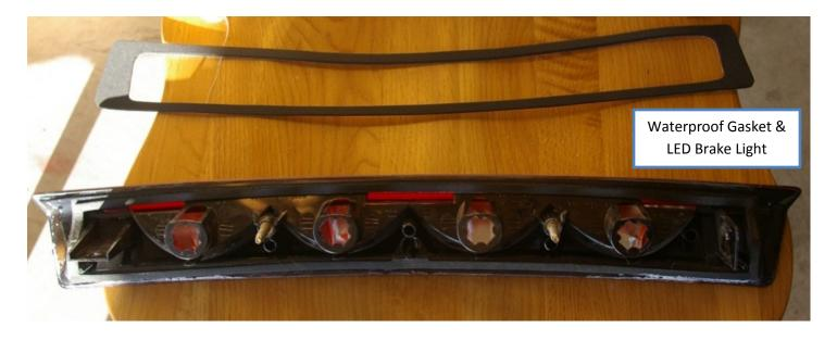
7. Now it's time to attach the old wiring harness to the new LED brake light. Fasten the last socket with attached bulb to the end of the new brake light. Continue to attach each new LED plug into their corresponding sockets.
