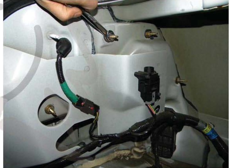
8. Remove the (4) 11mm nuts
