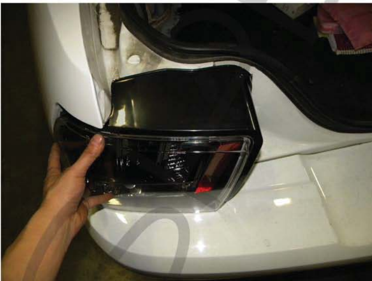
15. Place the LED tail light into the stock location
