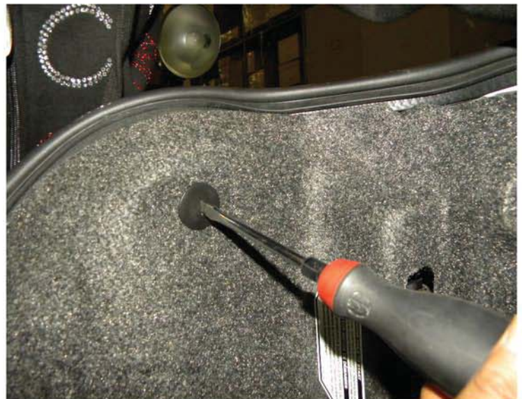
4. Remove the plastic flat head clip
