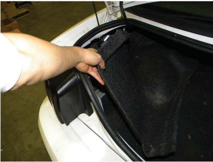
17. Replace the side trunk liner
