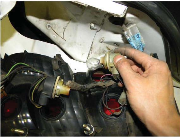
11. Leave the reverse light bulb in the socket please see the " L.E.D. tail lights installation instruction" If your tail lights don't have L.E.D. You can skip the installation instruction.
