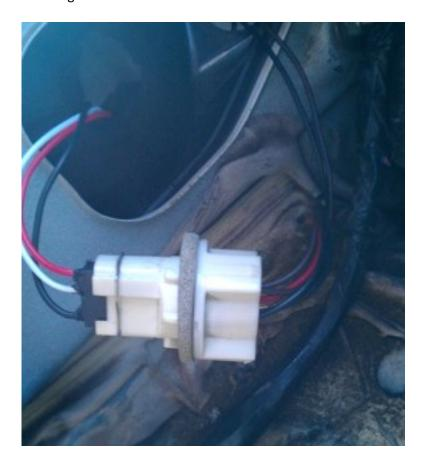
15. The round brake light socket will connect with the black and red LED wire plug. Again, match up the red of the LED wire to the red wire of the cars socket. Then install into the proper location on the taillight.
