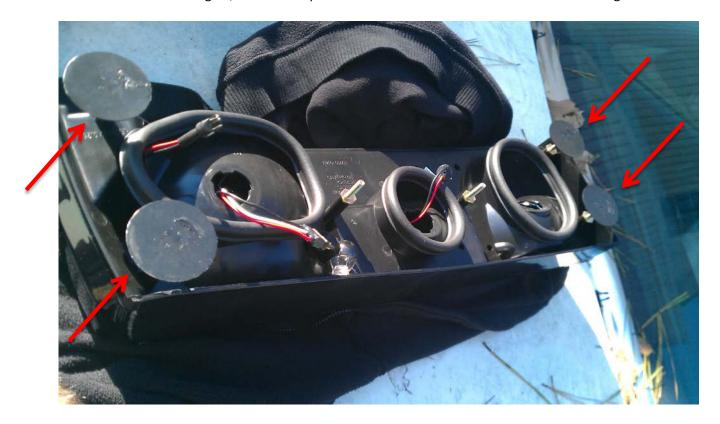
11. Match up the holes on the back of the car to the new taillights as shown in the picture below and push them in place. Reinstall the (6) nuts onto the new taillights being sure not to over tighten the nuts.
