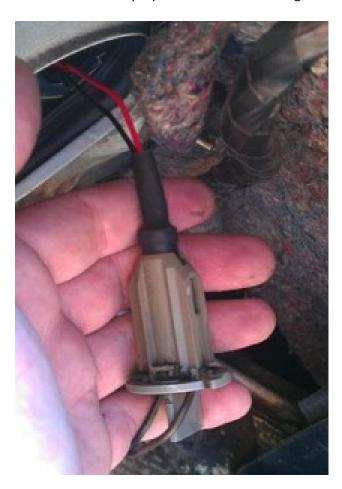
14. The brake light socket held in with the metal tab connects with the red, black and white LED wires. Match up the red wire on the LED with the red wire on the cars socket and push it in as shown in picture below. Then install into proper location on taillight.
