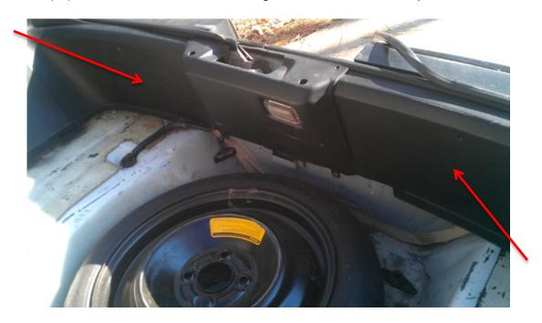
5. Remove the clip for the hatch light attached to the back side of the plastic interior pieces, see image below.
