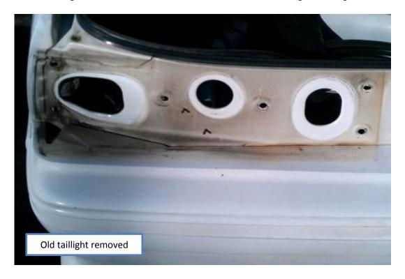
10. To install the new tail lights, remove the plastic covers on the bolts on the back of new tail lights.
