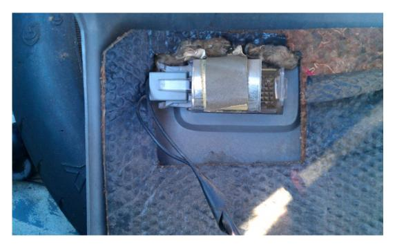
6. Remove the light bulb sockets from the back of old tail lights; they just turn and pull out, see image below.
