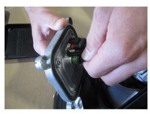
**Step 2:**Remove the plastic bulb cover and the HID bulb (Be very careful not to touch the actual bulb once removed)
