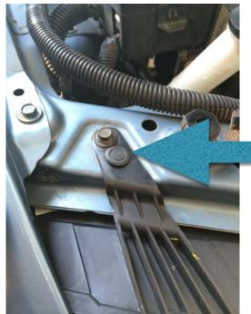
CAUTION: REMOVE THE BOTTOM BOLTS FIRST AND THEN THE TOP SO YOU CAN HOLD THE HEADLIGHT WHILE YOU UNPLUG THE HARNESS
