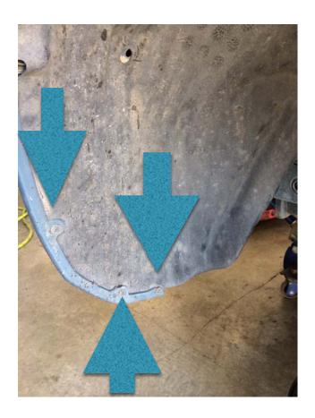
4.) Using the screw driver or screw gun with the Phillips #2 head, remove the 3 screws along the outer edge.
