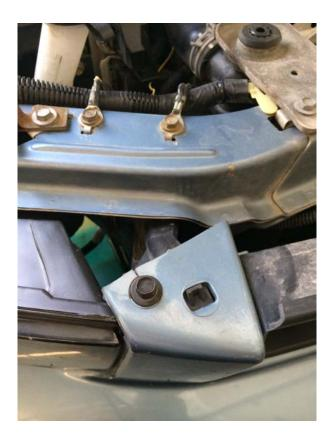
—If you have a GT or Fog lights Installed in your car, unplug the fog lights before completely removing the bumper—
