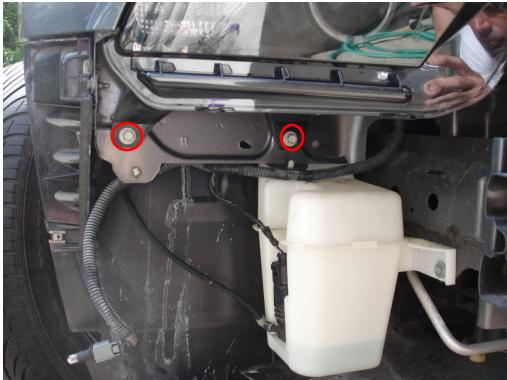
**12.** After removing the headlight from its attachment position, twist the bulb sockets to release them from the headlight and set the headlight aside. Disconnect the stock headlight bulb at the harness connector and set aside. If your state law requires or you prefer, remove the stock clear turn signal bulb and replace with the supplied amber bulb. Repeat this step with the other headlight.
