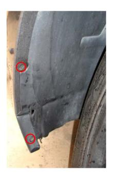
**3.** Lay a towel or blanket underneath and parallel to the front bumper. Lay on your back facing up and remove the (4) 7mm bolts from under the front of the bumper which attaches to the black plastic splash guard. Nothing will be completely freed at this time, but this will release the bumper from underneath.
