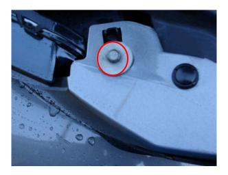
**6.** Carefully grab and pull the upper corner edge of the bumper next to the wheel well. The bumper is snapped into place here and will pop loose with moderate pressure forward. Work the bumper free, but leave it hanging in place.
