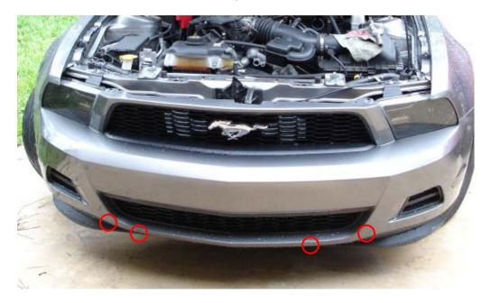
**4.** Using a flat head screwdriver and/or needle nose pliers remove the (8) plastic retaining clips holding the plastic radiator cover in place. Lift the plastic radiator cover off and set aside.
