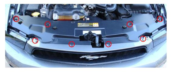
**5.** Remove the (2) 8mm bolts attaching the bumper cover up top. The bumper is still held on by the plastic tabs directly above these bolts. Leave the bumper hanging on these tabs at this time as this will prevent the bumper from dropping.
