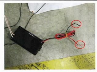
Step6. There are 2 wires on the IV box for the parking lamp: black is negative, red is positive. Please note that the IV box has a high voltage and make sure it is turn off while handling the wires.
