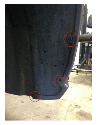
5. Remove the two outermost nuts on each side of the bumper. They are shown here:
