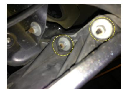
Be sure to only remove the two pictured above. When these are removed, pull the bumper off of the studs, and be careful not to scratch it.
