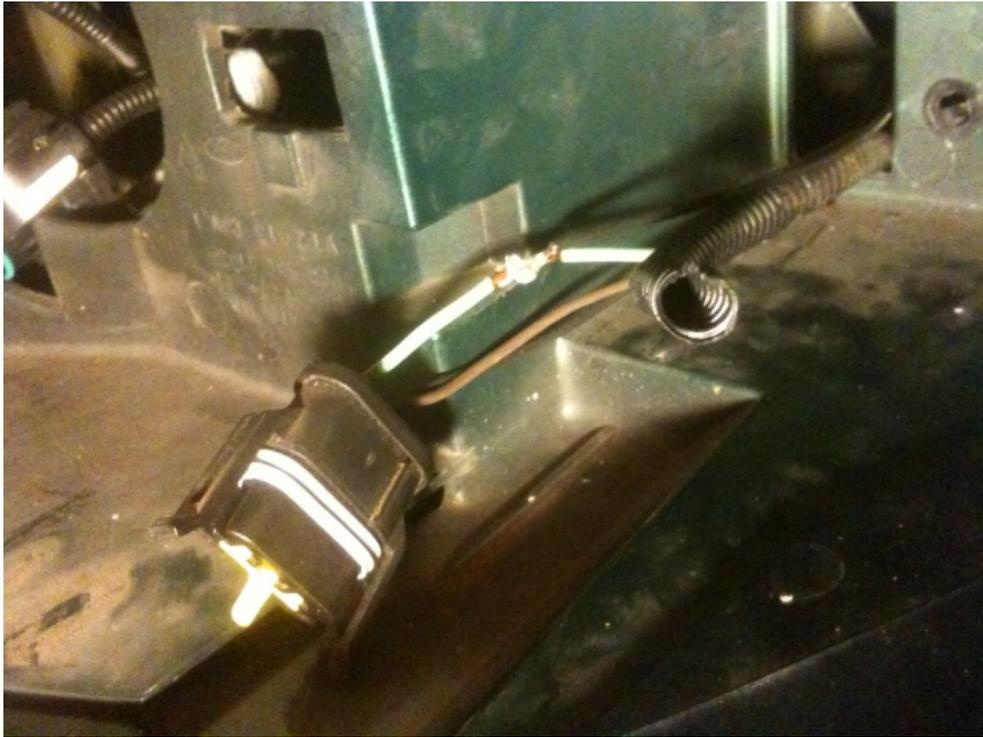
7. After the solder has cooled, tape the connection with electrical tape and replace the plastic wire protector cover. Put the turn signal bulbs back into the headlamp and turn clock wise till clicks into place. Reconnect the headlights and turn signal connectors. Before putting the headlamps all the way back in, test the LED's.
