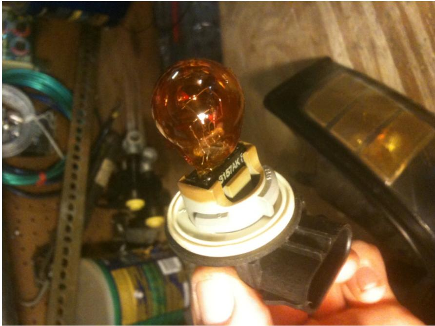
3. Remove the bulb by pulling straight out. Then take the new LED bulbs and replace by sliding straight into the socket
