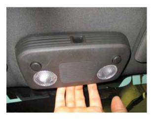
Step 3. Note: Some LED bulb fit snuggly which can potentially push the bulb socket out of the housing while installing the bulb, if this happens simply removing the housing and hold the bulb socket while you push the bulb in through the lense opening
