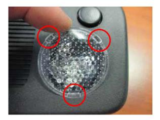
Step 1. Use a small flat screw driver to carefully pry up the lens cover. Note the orientation of lense to the housing.
