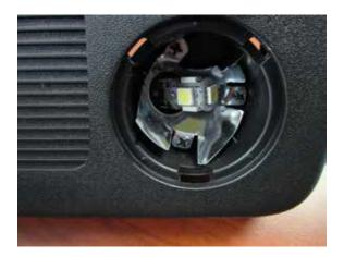
Step 2. Remove the factory bulb and instsall the new LED bulb.
