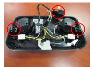
Step 4. Note: The 2 clips that hold the housing to the headliner. Disconnect the plug to remove entirely.
