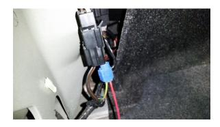
**STEP 5.** Using the second supplied wire splice connector, wire the other side of the load equalizer to the ground circuit.
