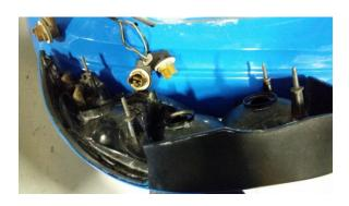
**STEP 3.** Identify the signal wire (Green / orange) and ground wire (black) before the harness is connected.
