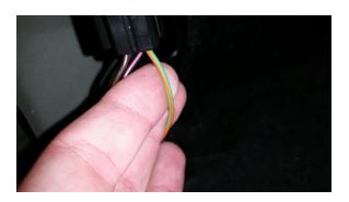
**STEP 4.** Using the supplied wire splice connectors, wire one side of the load equalizer into the signal wire.
