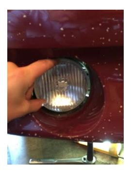
Step 5: Once aimed fully tighten the nut.
