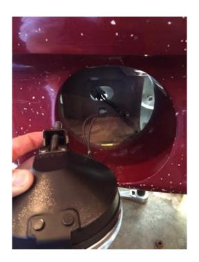
Step 3: Thread on the new 19mm nut onto the fog light stud. Do not fully tighten Step 4: once snug aim the fog light in your preferred direction.
