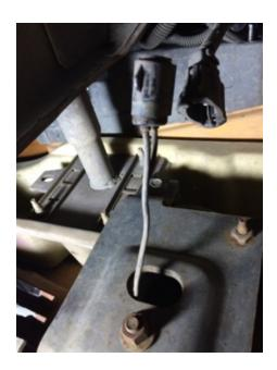
Step 2: Using the 15mm socket remove the nut holding the fog light in place.
