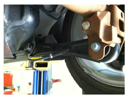
3. Use a small screwdriver or your fingers to pry the clip out of the e-brake line mount, the clip is silver in color but comes out easily. When you have removed the clip, use the small pry bar to lift on the metal arm that keeps tension on the e-brake line so you can disconnect it and pull it through the factory LCA.
