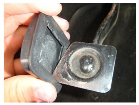
6. Next, bend the top rubber clip over the pedal, followed by the right clip, and finishing with the bottom clip. Push on the cover until you are satisfied with how it is sitting on the pedal, and finish with sitting on the seat and pushing on it with your foot in order to test it out.
