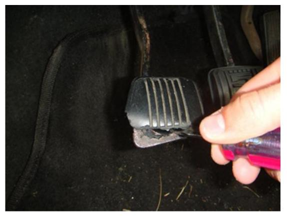
4. You'll notice below that the bottom clip on my clutch cover broke in the removal process. Taking your time is a sure-fire way to keep your old cover's clips in place.
