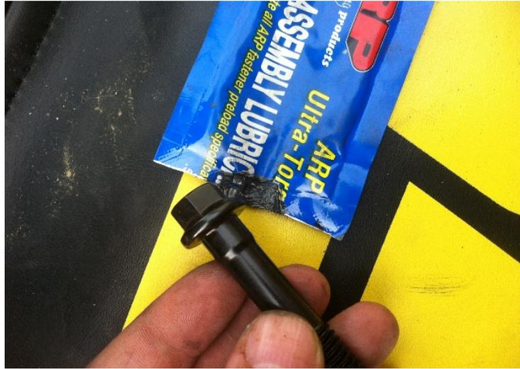
Photo 2: Preparing head bolts with assembly lube
