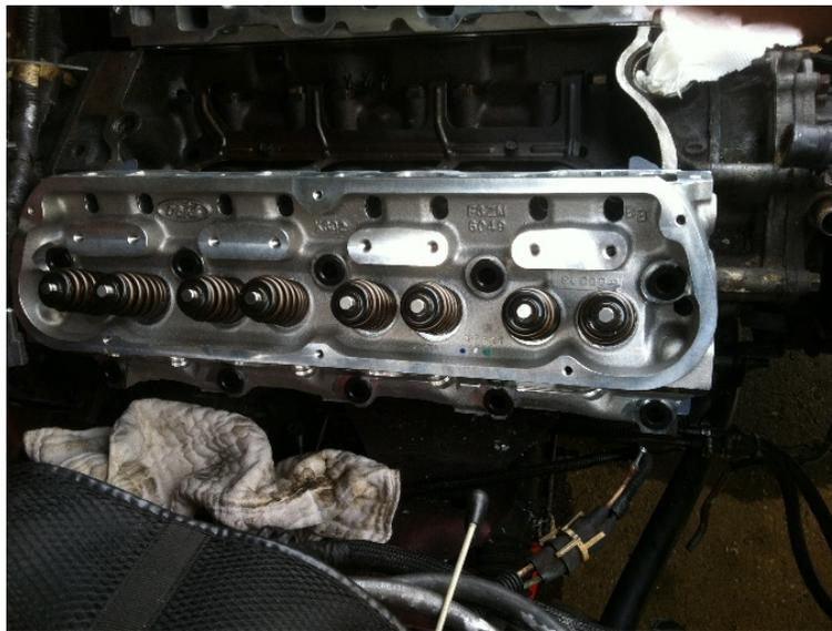
Photo 1b. View of all step washers in place on cylinder head.
