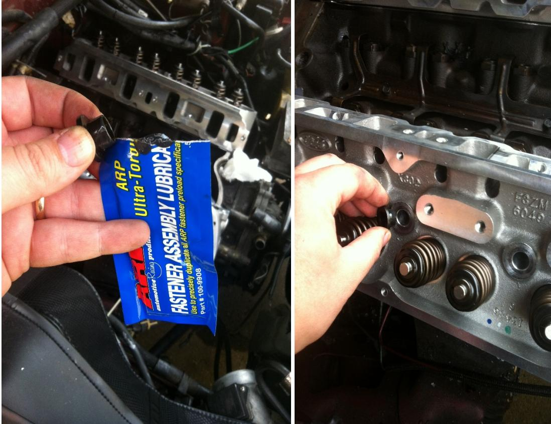
Step 1. Photo 1a: Applying assembly lube to step washer and mounting on cylinder heads.
