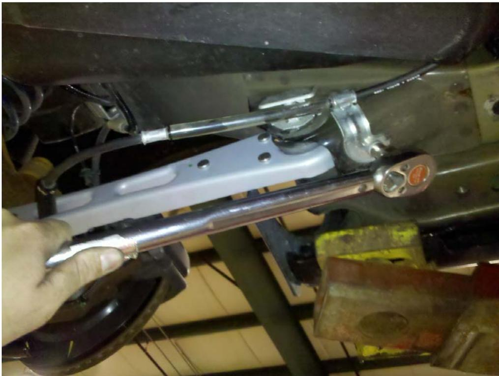
18. Installation of Passenger side LCA uses the same steps as the driver side.
