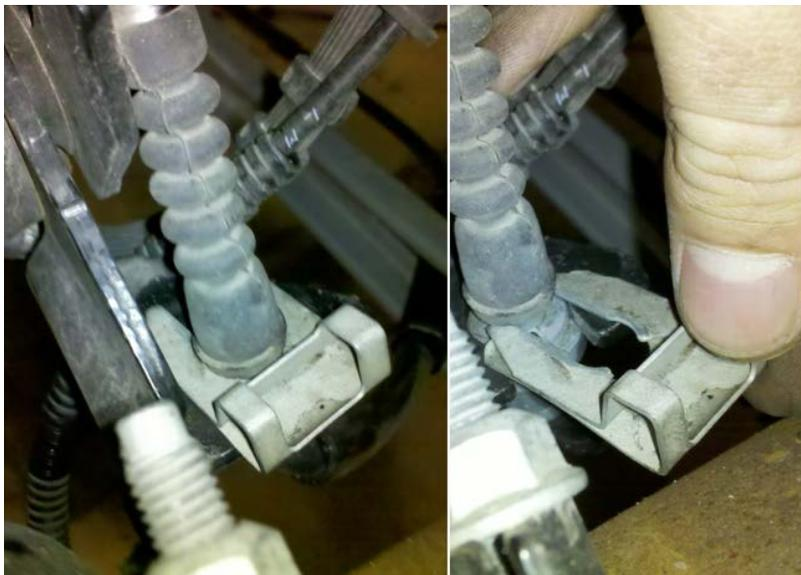
3. Remove the end of the emergency brake from the bracket and then feed the cable through the LCA.
