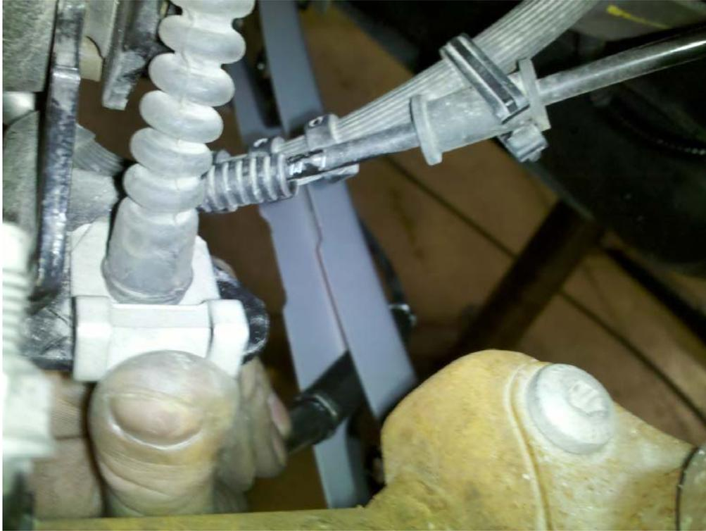
17. Reinstall the emergency brake cable bracket.
