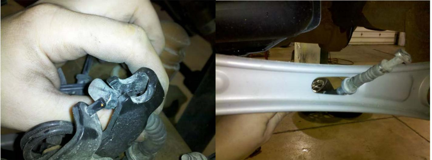
4. Using the 18mm wrench, remove the front bolt from the control arm.
