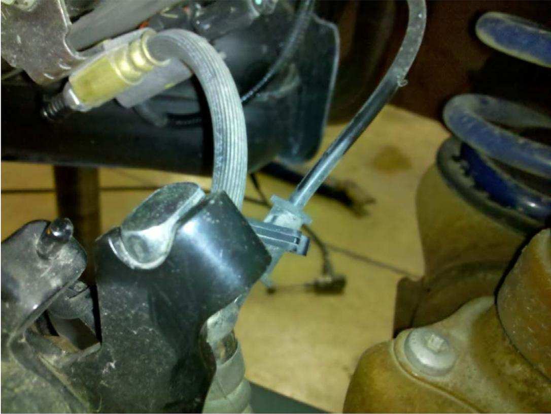
15. Reinstall the base of the emergency brake into its position on the caliper bracket.
