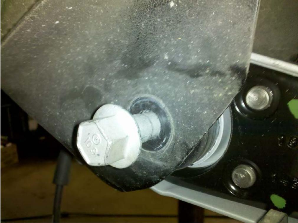
11. Using a torque wrench with an 18mm socket, torque rear bolt to 129 ft-lbs.
