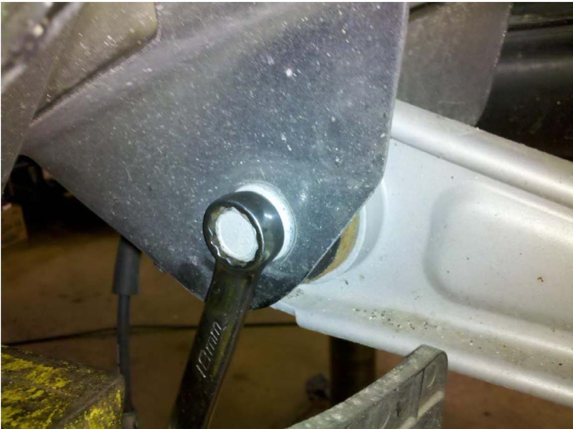
5. Once the bolt is out, the nut will still be in place. Rotate the nut clockwise to remove it.
