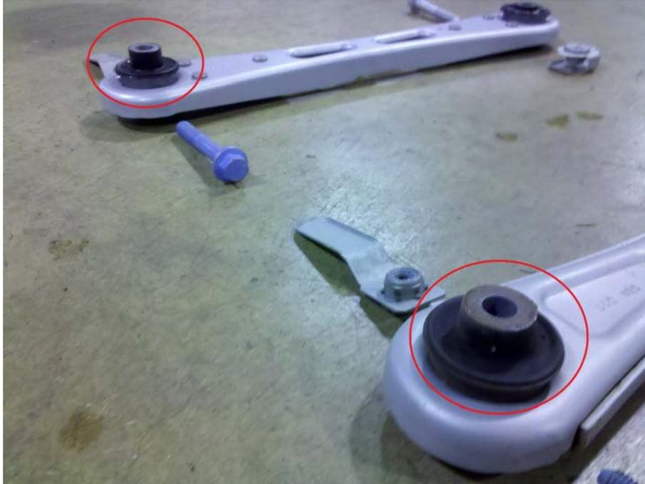
8. Take the new arm and place it in the bracket on the car, starting with the back bolt. Using the new blue bolt and new nut with handle, start the bolt from the center of the car and feed it through the hole towards the outside of the car. Before sliding it all the way through, position the nut accordingly, so the arm is against the rear end. This will hold the nut in place while you tighten the bolt. **\*Do not tighten bolt all the way, just enough to keep the nut in place.**
