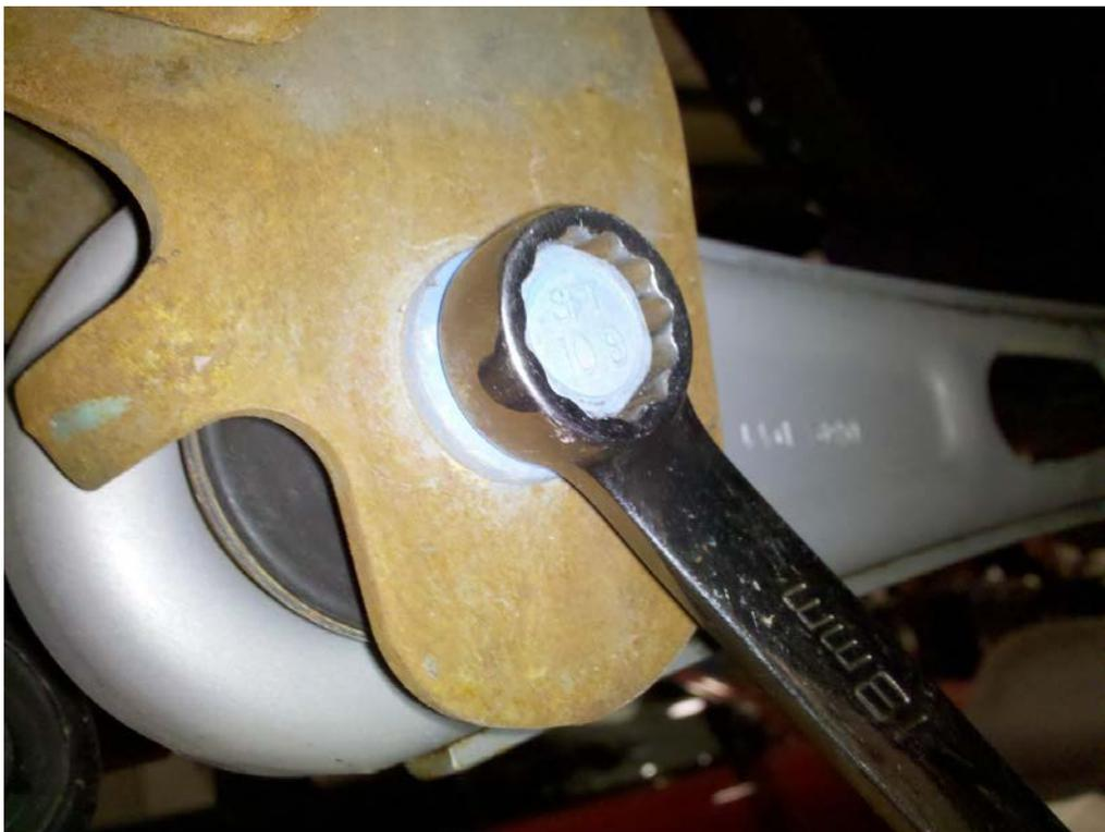
7. Notice the orientation of the factory control arm. At the rear, the spacer on the bushing is wider on the one side. This side should face the center of the car.
