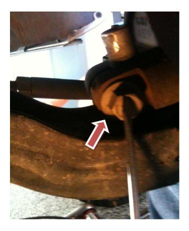
5. Carefully separate the steering knuckle from the ball joint and control arm. You will need a small pry bar for this. It may take 2 people with a pry bar on both sides of the ball joint. If pry bars are not available, you may use a large screwdriver or the flat end of a tire iron.
