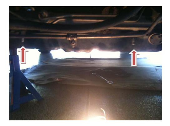
7. Pull the steering gear forward about 6 inches to allow for enough clearance to remove the forward pivot bolt.
