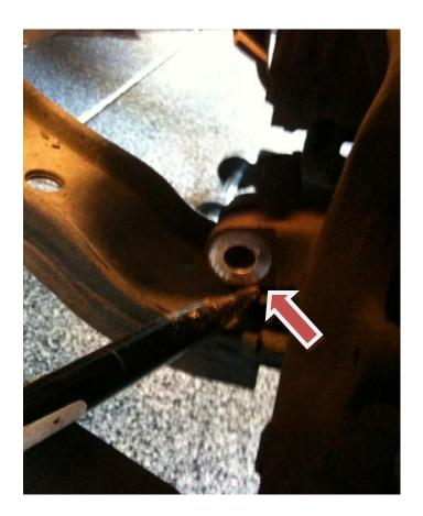
6. Remove both steering gear mounting bolts from cross member (18mm):
