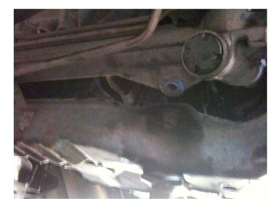
8. Loosen forward pivot bolt and remove with an 18mm socket. There is no need to hold the nut as it will not move; just turn the bolt head.
