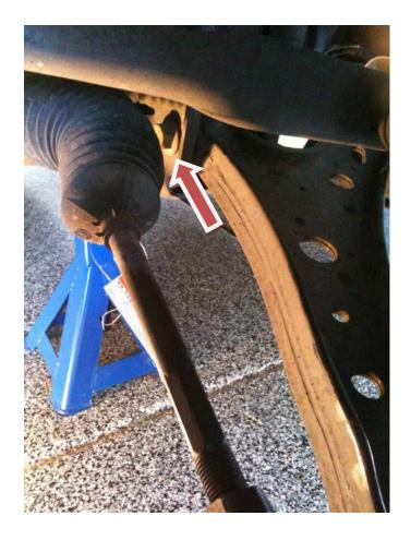
9. Remove the rear mounting fasteners (flag bolts) with a 21mm wrench.
