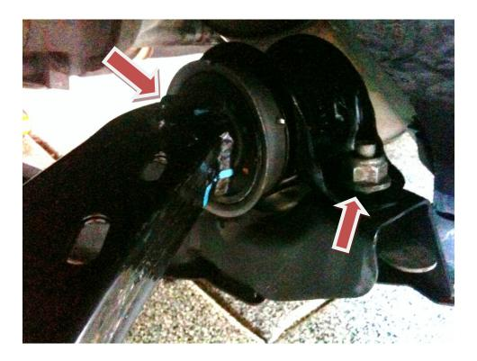
**NOTE:** This picture was taken after installation of new LCA. When removing the stock control arms, these bolts will be facing the opposite direction with the nut on the bottom. If you choose, you may reinstall the flag bolts like this. The rear bolt is hidden in this picture, but looks the same – arrow pointing to general location.
