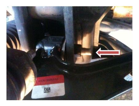
3. Insert the ball joint into the steering knuckle. Ensure that the groove on the ball joint stud is aligned with the hole for the steering knuckle pinch bolt for proper installation. It may help to raise the control arm with a jack to push the ball joint up. If you do this, place the jack directly underneath the ball joint.
