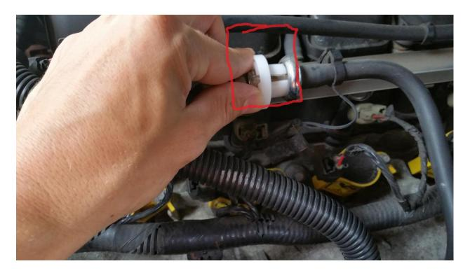
7. Disconnect the electrical connector and the vacuum hose from the Fuel Raul and Pressure and Temperature (FRPT) sensor. Both components are circled in the picture directly below.
