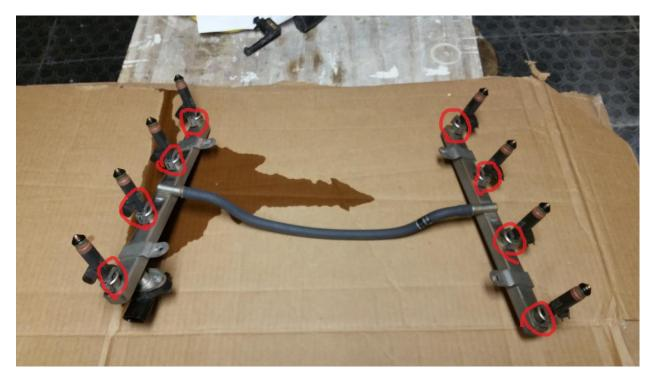
13. Remove each fuel injector retaining clip and then the injector from the fuel rails. If an injector sticks in the fuel rail, you may gently wiggle it side-to-side while simultaneously pulling on it. The injector clips are circled in the picture above and have been removed in the picture directly below.
