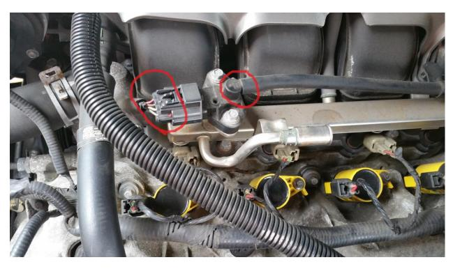
8. Remove the intake manifold plenum (if equipped – this is referring to the decorative intake manifold cover) by gently pulling it up and out of the engine compartment. You may need to loosen the top throttle body bolts to release the plenum.
