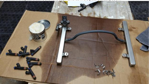
14. As you can see in the picture above, I decided to quickly polish the metal fuel rails with a wadding metal polish that I typically use on my exhaust pipes. Other metal polishes may be used, just read the container and determine whether it is an appropriate product. This step is optional.
