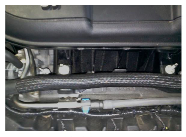
16. Reinstall the **Throttle Body** with the **(**4) **bolts** (**8mm**) along with its **electrical connector**.
