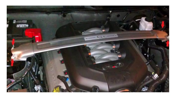
2. Remove your **Intake Cover** simply by pulling up on the cover and unsnapping it.
