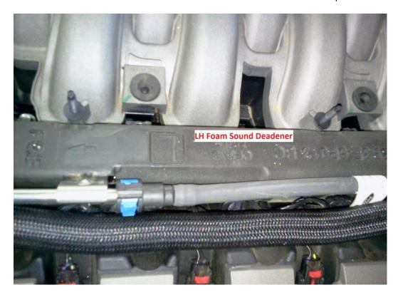
10. Remove the (4) Fuel Rail Retaining Bolts using a 10mm socket and an extension. Unplug all (8) of the Fuel Injector electrical connectors.
