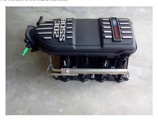
Finger tighten the 6 Intake Manifold retaining bolts and the 4 Fuel Rail retaining bolts, then torque them to 89 inchpound in the following respective sequences:
