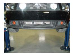
STEP 15: Clip the ambient air temperature sensor back onto the lower grille insert.
