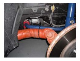
STEP 20: Slide the brake hose over the new backing plates and secure with provided hose clamp.
