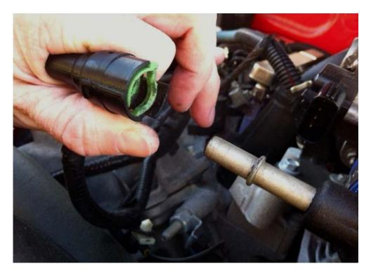
5. Remove the Mass Air Flow Sensor (MAF sensor) in the same manner as the TPS and Throttle Motor Harness. The MAF sensor is located on the factory air hose near the air box.
