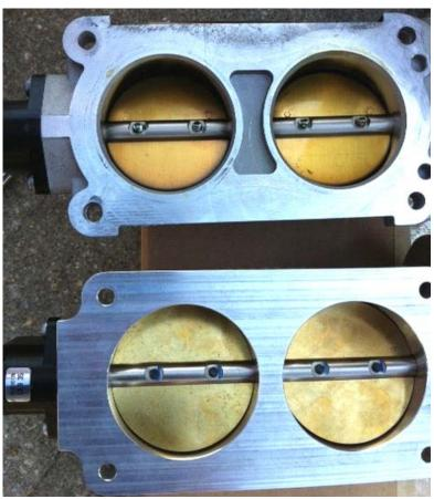
12. Slide the FR throttle body onto the lower manifold studs. Reinstall and hand-tighten the 8mm top studs.
