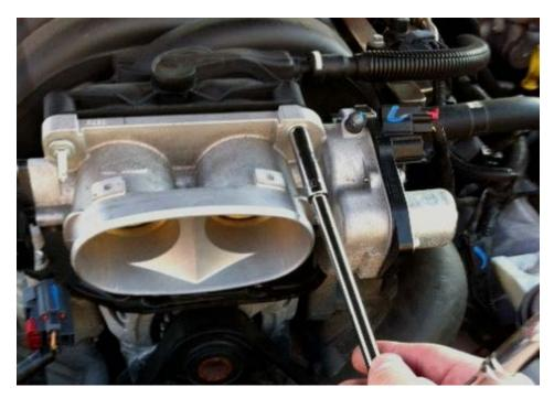
\*If the vehicle is equipped with an engine cover, this must be removed by (2) 8mm nuts on the top studs of the throttle body. Pull the rear of the cover off the (2) studs near the fuel rails. Pull forward and slide the cover off the throttle body studs.
