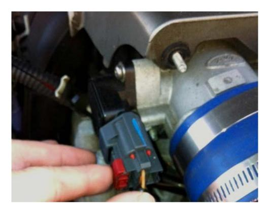
3. Disconnect the throttle motor harness on the driver side of the throttle body. Again slide the red clip back and press on the black tab to pull the harness free of the motor housing.
