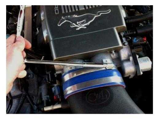
7. Pull the air hose fittings free of the throttle body and air box; set the air hose aside.
