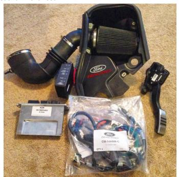
This installation guide assumes that your 4.6L 3V engine is already installed in the vehicle and all mechanical systems, such as transmission, clutch, exhaust, charging, cooling, power steering, and fuel pump and lines are already complete and installed. It is also assumed that the factory ECU and related harnesses are removed.
