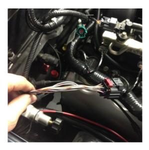
14. Pull back the tape and loom for the connectors to expose the wires to cut. Make sure to give yourself at least 2" of wire from the connector.
