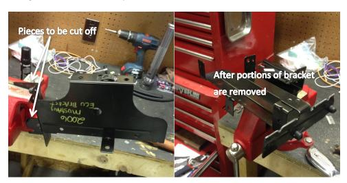
8. Using an appropriate metal cutting tool, remove the portions of the PCM bracket. (left) Remove any sharp edges.
