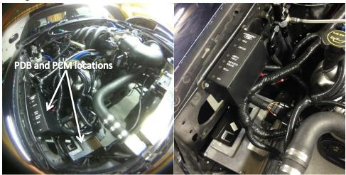
7. A factory PCM bracket (not included) from a 05-09 Mustang will be slightly modified to make the mounting of the PCM much simpler.
