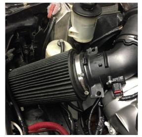
5. The long filter provided just squeezes into the area where the battery usually is on a Fox body. Connect the mass air flow connector.
