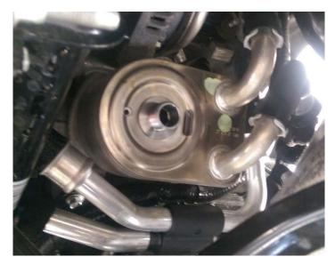
Once the cooler assembly is in all you need to do is connect the hose assembly to the lower radiator hose.
