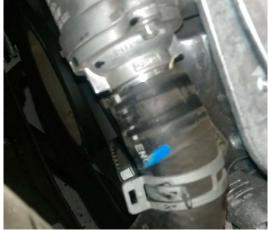
I closed the radiator drain plug at this point (after it was not dripping anymore) and moved the bucket to the other side to catch any remnants in the hose. There was maybe a cup or two that came out when I pulled the bottom of the hose off, which is the next step.  $\odot$
