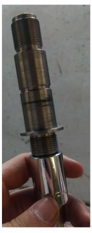
Be sure to start the center post by hand, you do not to strip the threads on the engine block. There are some alignment tabs on the back of the assembly to make sure it is aligned, sorry I didn't get a picture of that.
