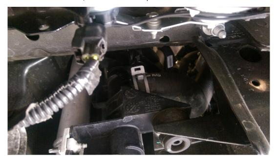
To pull the bottom hose off you need to do the same thing, squeeze the clamp, and slide it off of the radiator. Once the clamp is off you need to squeeze and slide the hose to get it off of the radiator, just like you did with the top part.
