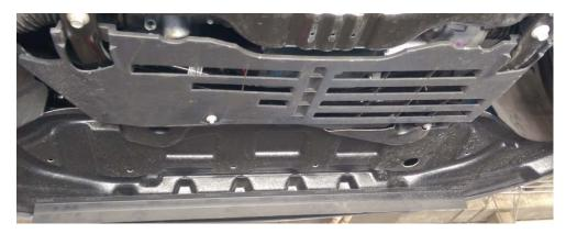
After the bottom panels are reinstalled you can lower the car down and put the top parts back together, mainly the airbox. Once everything is installed it is time to put the fluids back in.
