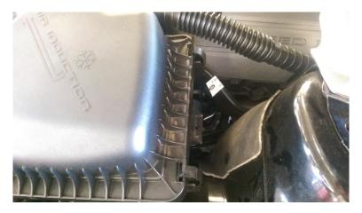
Below is the screw, it is on the driver's side of the airbox. After this screw is removed all you need to do is remove the sound tube by pulling it up, pulling the airbox up, then back towards the driver's seat. It is only held in with rubber grommets. The reason to remove the complete airbox it is to get to the top of the radiator hose clamp easier.
