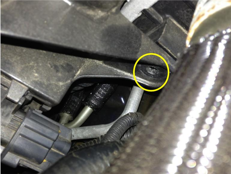
16. Use a small flat-tipped screwdriver and install it into the plug until you feel it push on the locking lever. Twist the screwdriver while pulling on the radiator fan plug to disconnect it.
