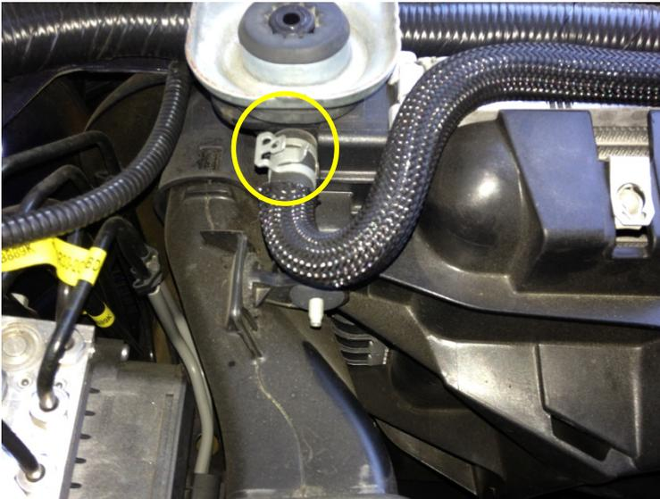
11. Use a 10mm socket, extension, and ratchet (or speed handle) to remove the reservoir tank bolts.
