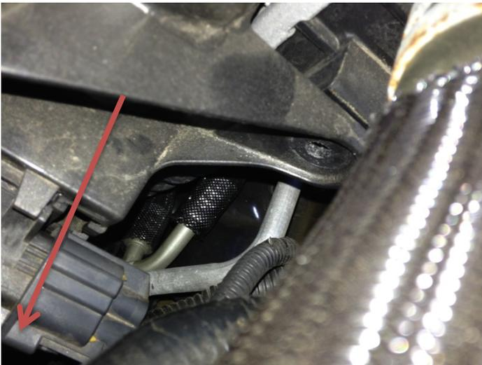
17. Remove the factory fan assembly by pulling it up, alternating between left and right until the fan clears the vehicle. Essentially, there were three bolts holding the stock fan in place (as shown by the yellow circles). The new fan only uses two bolts. The mounting boss for the bracket with hoses from Step 14 is shown by the red arrow. The new fan does not have this mounting boss.
