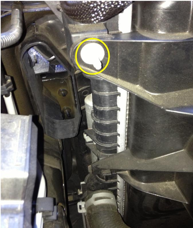
14. If equipped, use a 10mm socket and ratchet to remove the hose bracket bolt at the bottom of the fan assembly. The SVT fan does not have a mounting area for this bracket and it will not be re-used. Cutting this bracket off is not recommended due to risk of damaging the lines which are attached.
