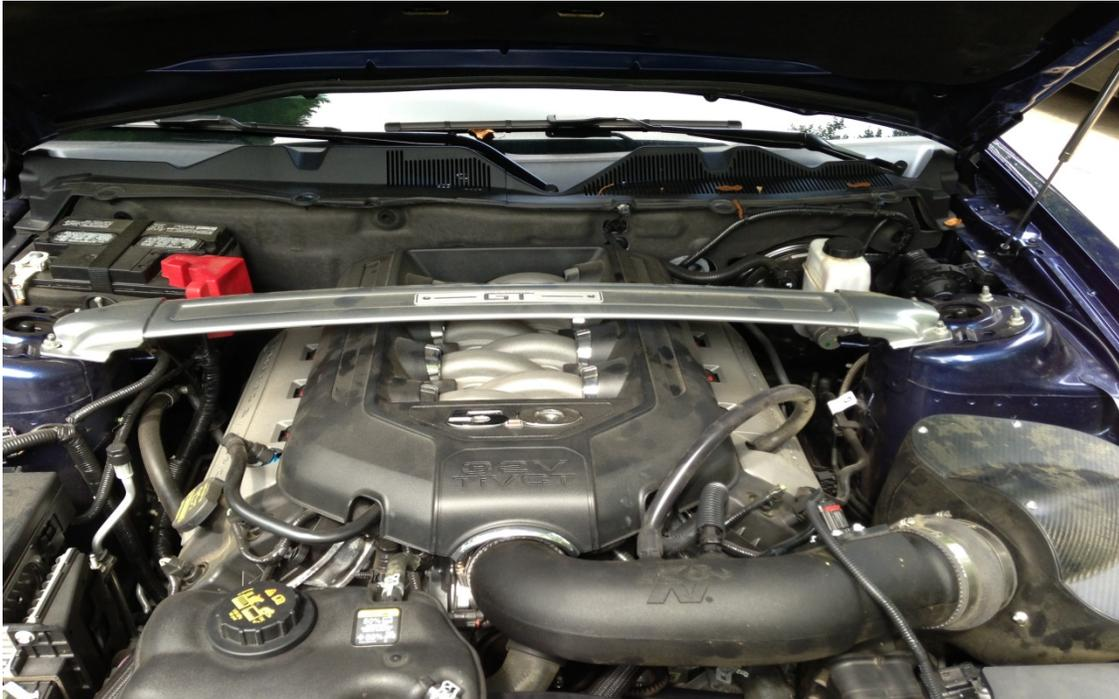
3. Carefully remove the plastic engine cover by gently pulling up at the front (radiator end) and both sides to unseat it from the grommets securing it to the top of the engine (4 places).
