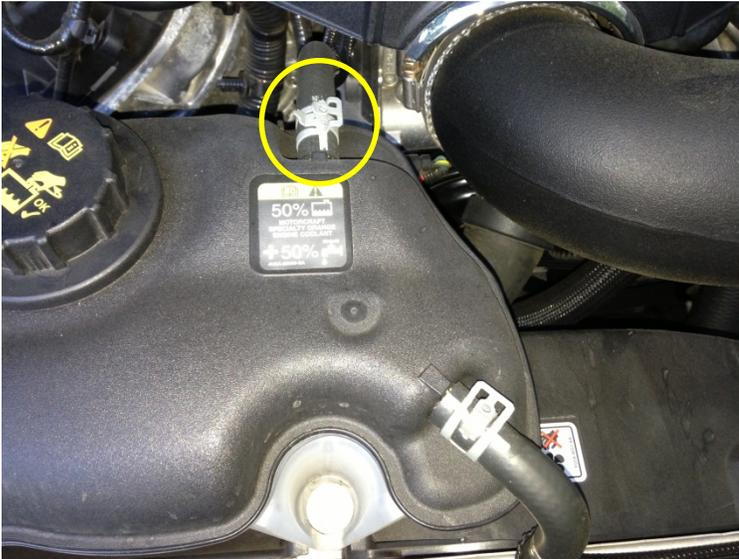
10. Use the slip-joint pliers to squeeze the small hose clamp going to the top of the radiator and use a slight twisting motion to pull the clamped hose away from the radiator. Use a plastic container to catch coolant if necessary.
