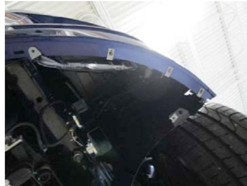
**STEP 35:** Install the new splitter into the fascia by aligning the splitter clips with the fascia. Gently push into place and verify the (6) splitter clips are securely attached.
