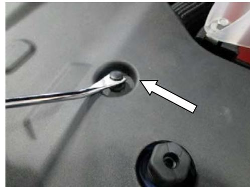
**STEP 15:** Remove the upper radiator close off shroud.
