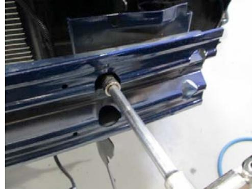
**STEP 22:** Insert the new splitter bumper bracket from the top side. Hang the bracket from the bumper verifying it aligns over the (2) remaining bumper bolts.
