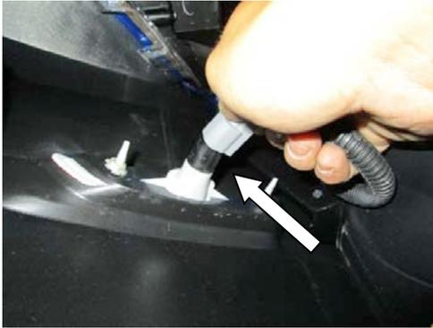
**STEP 14:** Remove the (8) push pins retaining the upper radiator close off shroud.
