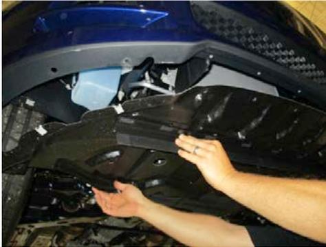
**STEP 5:** Remove the (2) bolts holding the production chin to the fascia.
