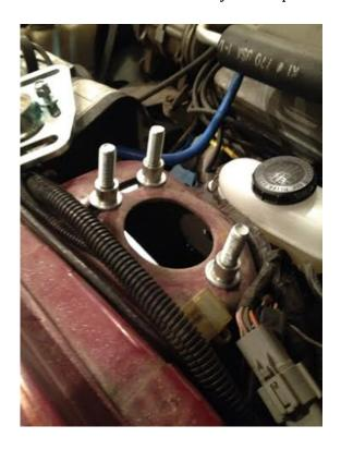
Step 4: Take the upper caster camber plate and meet it up with the lower plate. Slide it down onto the three studs.
