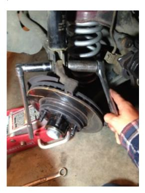
Step 13: With the two nuts removed, hold the strut with one hand and use the other to remove the two bolts that hold the strut to the spindle.
