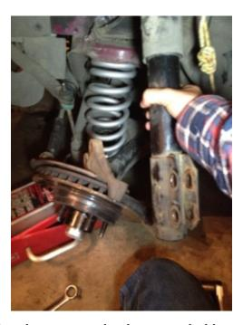
Step 15: With the 9/16 socket remove the three nuts holding the stock caster camber plates to the strut tower.
