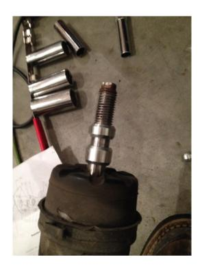
Step 8: slide the strut up through the caster camber plate.
