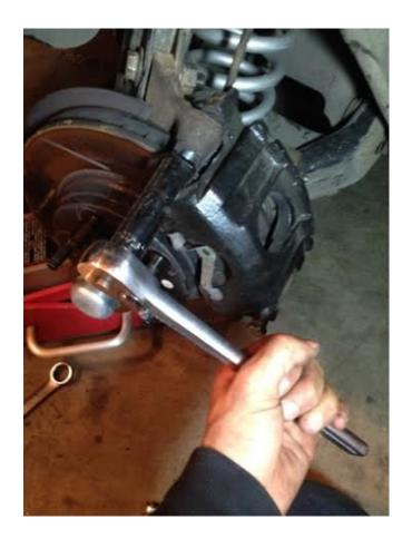
Step 16: Insert the two bolts and tighten using a 17mm socket.
