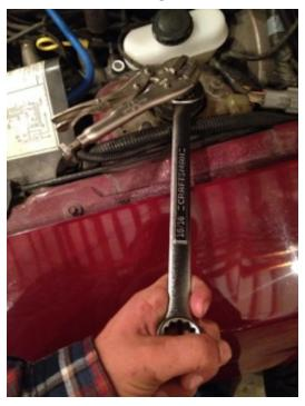
Step 11: While holding the vise grips take the 15/16 wrench and unscrew the nut holding the strut to the old caster camber plates.
