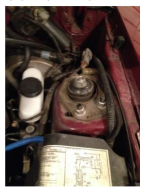
Step 9: Looking at the top of the strut from under the hood you will see a machined spot at the end of the threaded stud, Take the vise grips and clamp them on the end of the threaded stud.
