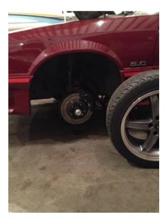
Step 6: With a 17mm socket remove the two bolts that hold the caliper onto the spindle. Repeat for both sides
