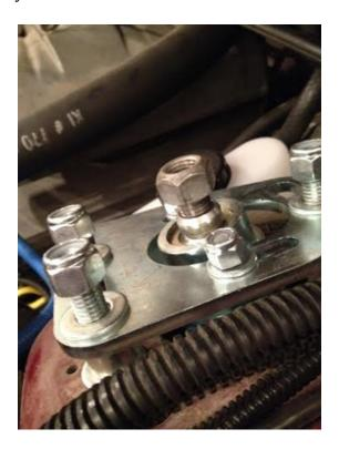
Step 10: Take the bottom of the strut and line up the two holes with the holes on the spindle and insert both bolts and thread on both nuts.
