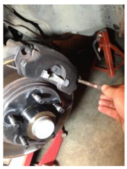
Step 7: Pull the caliper from the rotor and hang from a hole in the fender well with a bungee cord so the brake line is not supporting the weight.
