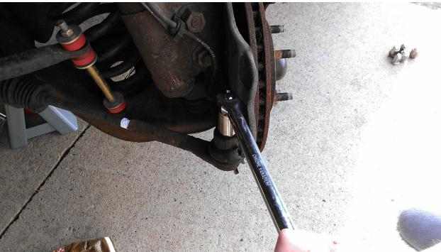
5. Mark on the inner tie rod shaft with tape and/or a marker where the old lock nut is so the new one can be placed in the same general position
