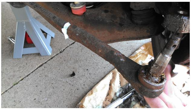
7. Loosen the lock nut with a wrench on the lock nut and a vice grips on the tie rod
