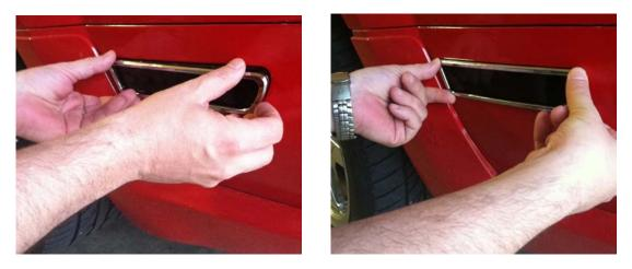
(4) Firmly apply pressure all around the trim and then allow to set ~6 hours at ~70F or ~ 20C.
