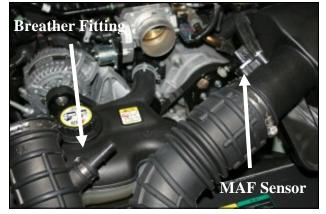
**5.** Using the supplied #20 torx bit, remove 2 factory screws, and remove the **MAF** sensor from the factory tube. (Save the **MAF** sensor for reinstallation in step #12). Next, using a pair of side cutters, remove the metal band that holds the plastic breather fitting into the factory air intake tube . Now remove the fitting from the tube, and save it for reinstallation in step #12.
