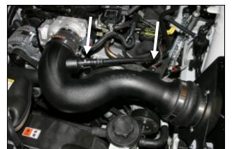
13. Install the intake tube assembly into the hump hose first, and then into the throttlebody coupler. Adjust for fit, and then tighten the three remaining hose clamps. Next, reconnect the MAF sensor wiring harness and lock the red tab. Now reconnect the factory breather tube to the factory fitting.
