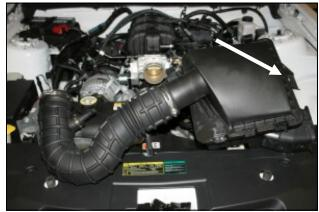
**3.** Remove the complete intake system as an assembly. Remove the factory grommet, and steel sleeve from the factory airbox for reuse in step #8.
