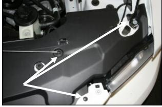
**6.** Using a flat blade screwdriver, pry up the center of the three plastic trim anchors that are shown. Once the center is up, then pry up the bottom half of the anchors up and out of the hole and save them for reinstallation in step #10.
