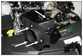
**8.** Install the filter adapter into the Cool Air Dam (#6) using three 1/4-20 button head bolts (#8), and three 1/4" flat washers (#9) as shown. Next install the factory grommet and steel sleeve removed in step #3 into the hole in the **CAD**.
