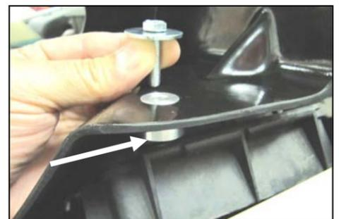
9. Slide the Aluminum Spacer (#14) underneath the CAD and into the hole as shown. Secure the CAD to the inner fender using the OEM bolt from step #3 and the supplied 1/4" Fender Washer (#15).
