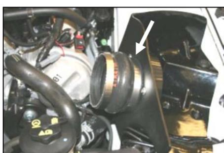
10. Install the hump hose (#4) on the filter adapter (#6), with two #72 hose clamps (#12). Tighten only the clamp next to the CAD.
