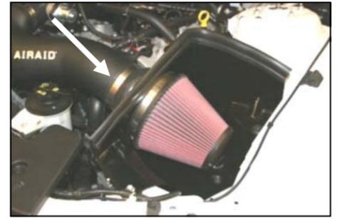
15. Install the Airaid Premium Filter (#1) onto the filter adapter, and tighten the clamp. Install the weather strip (#8) on the top of the CAD as shown.
