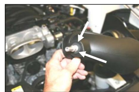
11. Install the supplied grommet (#13) and aluminum fitting (#16) into the Airaid intake tube as shown.
