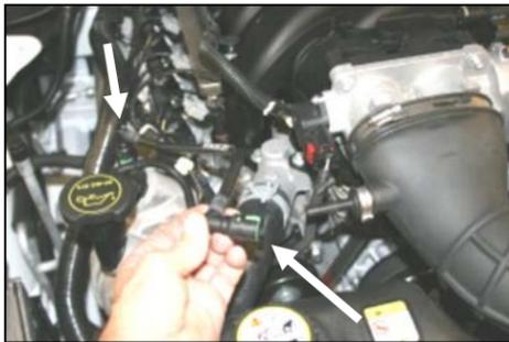
1. **Disconnect negative battery cable.** Push the green plastic tabs, and remove breather hose from vehicle. (Save for later use).
