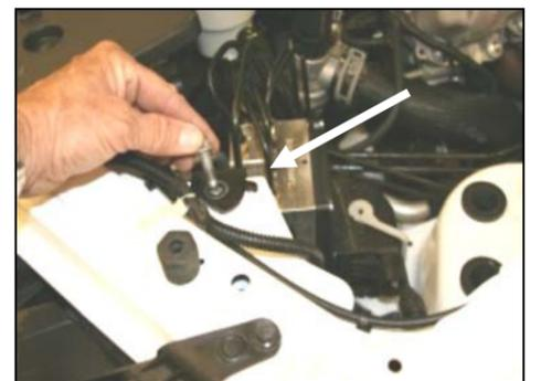
6. With a 10mm socket, remove and save the bolt from the anti-lock brake bracket. It will be re-installed later in step #9.
