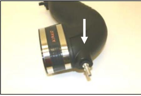
13. Install the oval coupler (#3) with two #72 hose clamps (#12). Tighten only the clamp closest to the aluminum fitting. (*Hint: For a clean look, locate the hose clamp tightening screws under the tube!*)
