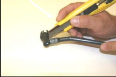
16. **VERY CAREFULLY!** Using a razor blade, cut the plastic tube off both of the factory breather hose ends as shown.
