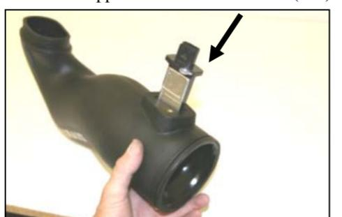
12. Align the two slots in the tubes, and install the factory mass air sensor removed from step #5. Make sure the screw holes line up, then install the two supplied button head screws. (#11). **DO NOT USE THE FACTORY SCREWS!!**
