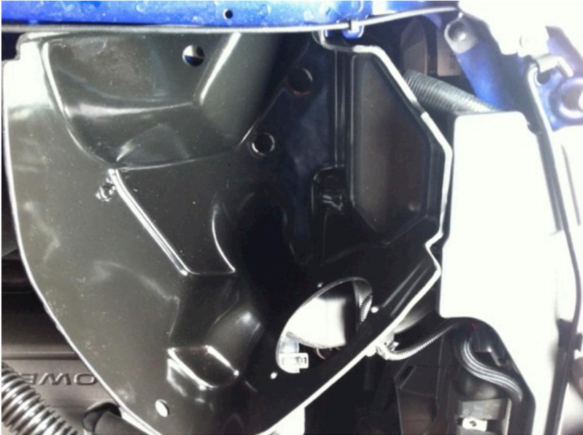
4. After you secure the heat shield, find the grommet with the 3 lock nut holes in it. Attach that grommet into the heat shield with the screws facing away from the vehicle. After that take the intake tube and fill the holes in it with the stock mass air sensor, the black rubber plug and the metal hose fitting.
