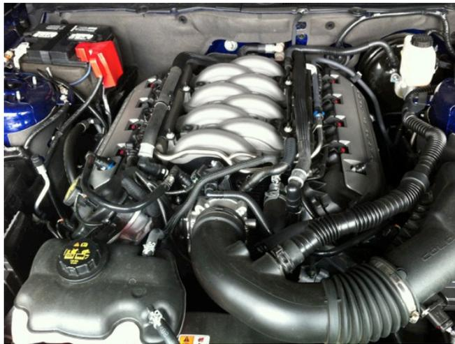
2. After you have the plenum cover removed you can now take off the entire stock air box and intake. Start by loosening the clamp on the intake tube that's attached to the throttle body. Then remove the bolt in the air box with the 10 mm socket. Once both are off disconnect the mass air sensor and the other 2 hoses attached with clamps and remove stock air box
