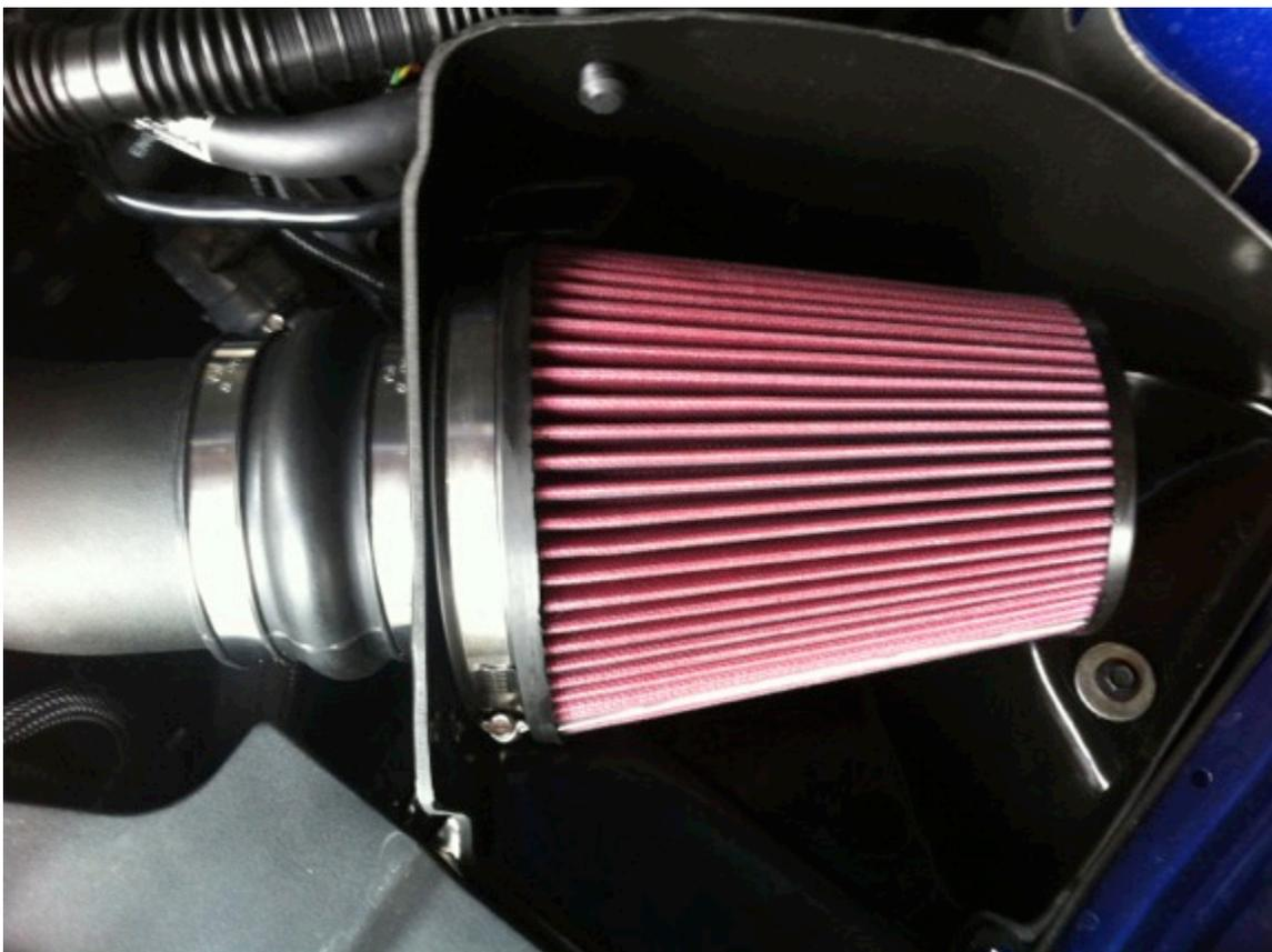
7. Once all tubes and clamps and grommets are in the correct place. Proceed to use the 8mm socket or flathead to tighten all of the clamps so that nothing will come loose from the pressure. Reattach the mass air sensor, vac line and sound tube to the new intake tube using the pliers and soapy water.
