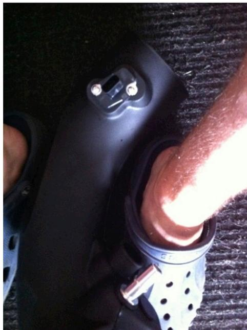
5. Once all pieces are attached to the intake tube, attach the tapered rubber grommet to the front of the tube with the medium sized hose clamp. Then attach the last grommet with the bubble in the middle to the end of the tube with a large clamp. After that secure the tapered grommet to the throttle body with a small clamp. (soapy water helps get hose and grommets together)
