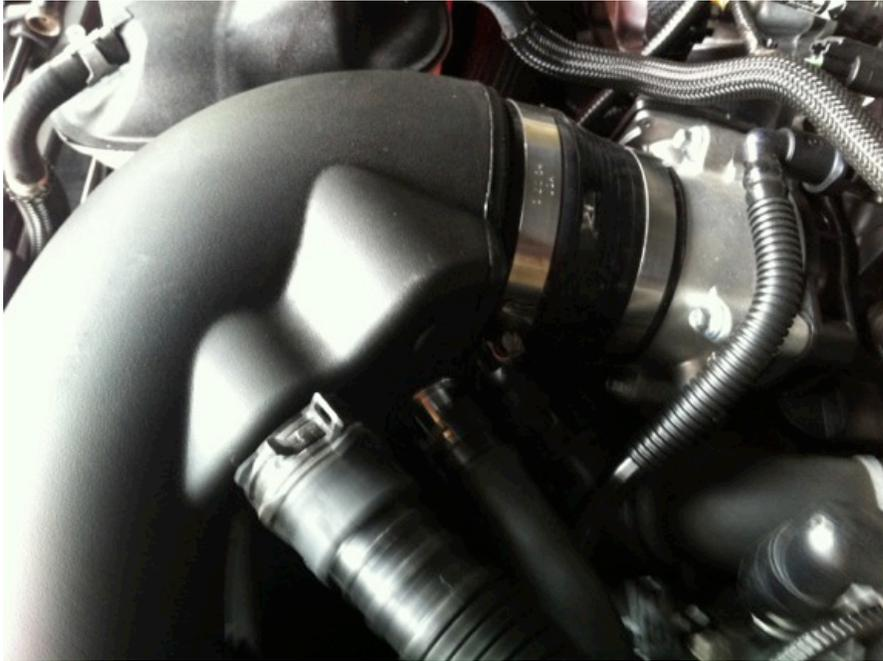
6. After securing the tube to the throttle body, attach the end of the tube with the big grommet to the other grommet that we secured to the heat shield using another large clamp. After that attach the air filter inside the heat shield with the last biggest clamp.
