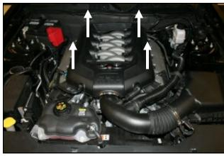
**Disconnect The Negative Battery Terminal!** 1. Remove the strut tower brace, if so equipped. Remove the Engine cover by simply lifting up, and set aside.
