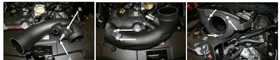
4. Install the Grommets and Fittings into the Airaid intake 5. Using the supplied Torx driver, remove the MAF sen- 6. Install the filter adapter (#6) using three 1/4-20 button tube (#2). A) All models will require the use of the 5/8" sor from the factory airbox and install the MAF sensor head bolts (#8), and flat washers (#9) into the Airaid Cool Fitting (#17) and the 5/8"Grommet (#19). B) Automatic into the intake tube using two provided 8-32x3/8" screws Air Box (CAB) (#3) as shown.
