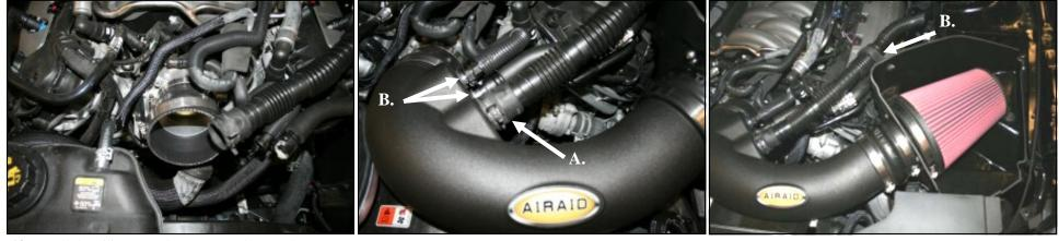
**10.** Install the Silicone Reducer (#5) and Hose clamps onto the throttle body. Place the #56 clamp (#13) on the Throttle body side of the reducer, and the #64 clamp (#12) on to the tube side.
