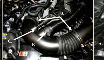
2. A) Loosen the hose clamps on the factory intake tube **B**) Squeeze the clamp and disconnect the resonator from the air intake tube. C) Carefully depress the hose lock tabs, and disconnect the crank case breather line and the brake aspirator line (if equipped, AT models only). D) Remove the factory intake tube.
