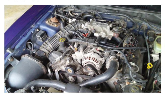
**Note:** Start with one coil pack and move to the next after completely finishing the previous one. It can help to start with one side and on one end and to move across as you go.
