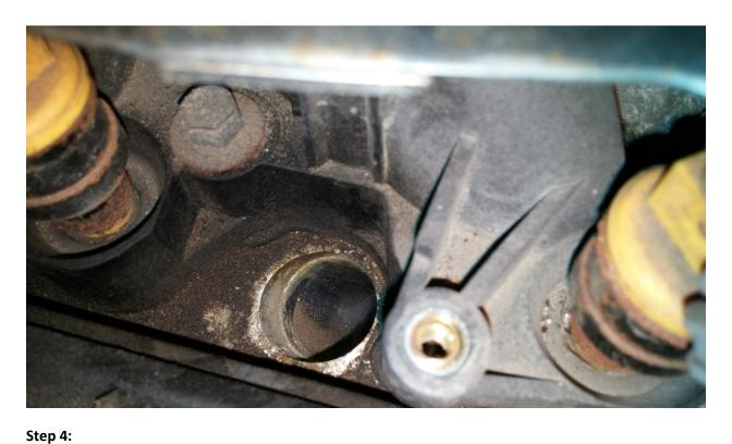
Place the new coil pack into the hole. Make sure it is seated down far enough and then replace the 7mm bolt. Tighten the bolt just to a snug feel leaving no vertical motion in the coil pack.
