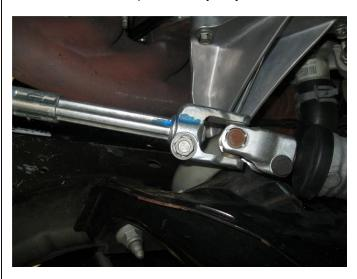
**Step 5.** Unplug the O2 sensor coupling for the header. When disengaging the steering shaft first mark both the shaft and the universal joint to ensure alignment on reassembly. Remove the retaining bolt and uncouple the steering shaft.
