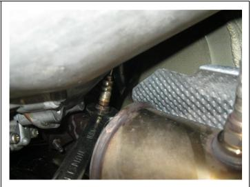
**Step 4.** Unbolt the O2 sensors in front of the catalytic converters. The H-Pipe assembly may now be removed.
