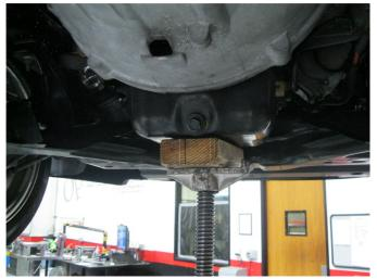
**Step 6.** Before removing the motor mounts support the engine with a jack.
