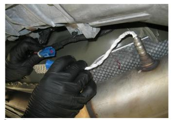
Step 2. Disconnect the rear O2 sensor plugs.
