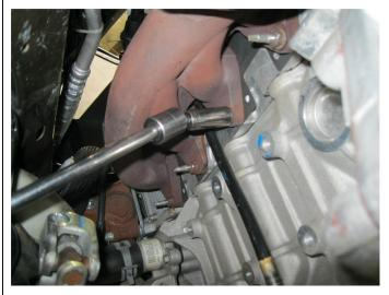
**Step 8.** The header nuts are now accessible, remove all eight and remove the studs too. The drivers side header may now be removed.
