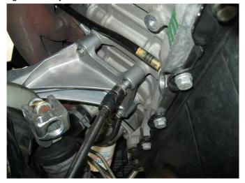
**Step 7.** The motor mounts may now be unbolted and removed.
