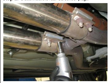
**Step 3.** Loosen the clamps attaching the H-Pipe assembly and unbolt the H-Pipe flange from the catalytic converters.
