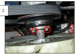
Loosen the (4) 11mm water pump / cooling fan bolts.
