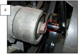
Attach a socket to the 18mm bolt, located in the center of the belt tensioner pulley and turn counter clockwise until the belt can be removed from all pulleys.
