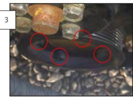
Loosen the (4) 9/16" crank pulley bolts in the crank pulley.
