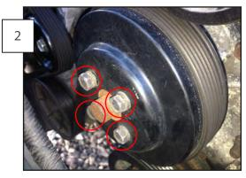
Loosen the (4) 1/2" water pump / cooling fan bolts.
