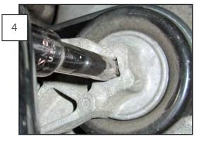
Attach a 3/8" socket extension to the square hole in the idler pulley and turn counter clockwise until the tensioner stops and the belt can be removed from all pulleys. Remove all hardware that was previously loosened.
