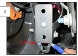
Insert a short cap head bolt through the relocation bracket. Insert the bolt into the upper sway bar mount bolt hole. Mark where the bracket ends, remove the bracket and cut off the lower side of the sway bar bracket.
