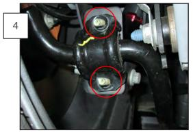
Reinstall the bracket with the short cap head bolt, secure it with a large washer and 1/2" locking nut.
