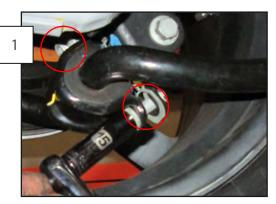
Remove the (2) 15mm sway bar mount bolts. Remove them by pulling the tab downward and sliding them toward the inside, while pulling them out by the threaded end.
