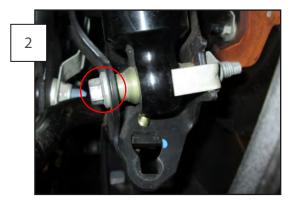
Remove the (1) lower shock bolt that holds the shock to the rear axle. Move the shock out of the way for the install.
