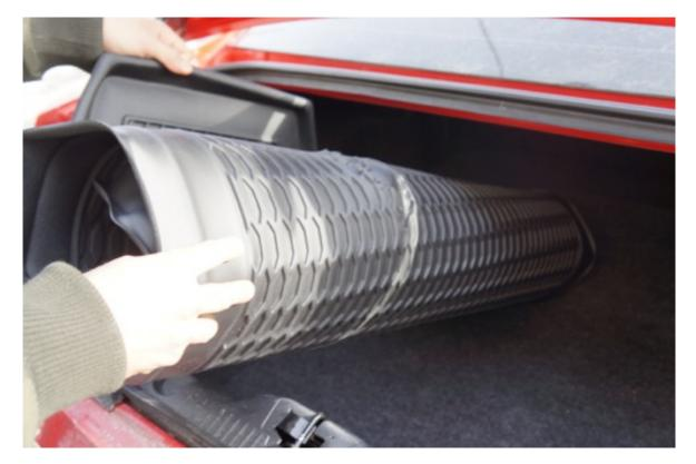
2. Roll out Ford Racing Cargo Area Protector from the center to right side of the trunk.
