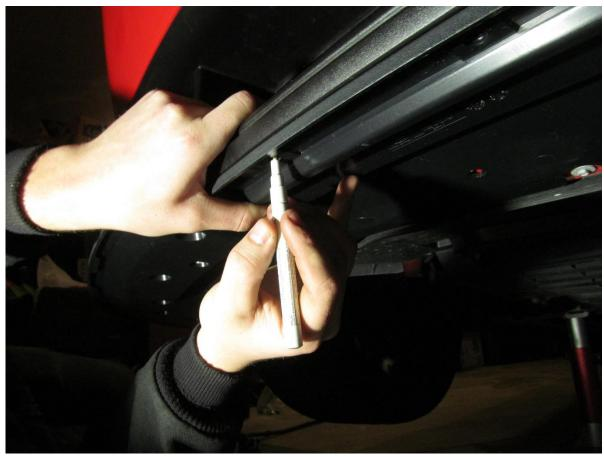
2. With the four holes marked it is time to drill them out. Start with a pilot hole using the 1/8" drill bit. Once the pilot holes are drilled go back and drill those holes out with the 3/8" drill bit.
