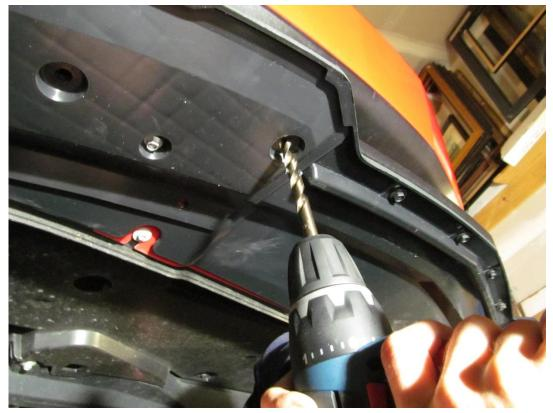
5. Now that all of the holes are drilled, remove the four bolts from the front of the Splitter installed earlier and lower the Splitter to install the rest of the clips on the bumper for the holes highlighted.
