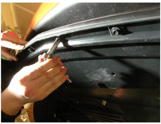
4. With the four front bolts installed the splitter is now in place. The rest of the holes can now be drilled out with the 3/8" drill bit right though each remaining hole of the Boss 302 Splitter.
