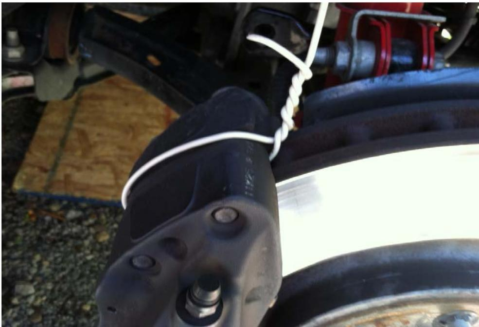
5. Now it is time to remove the two caliper mounting bolts. Use the 15mm socket and breaker bar to loosen the 2 bolts then continue to remove with 15mm and ratchet wrench. The caliper will pull straight off toward the cabin of the car. The brake pads may fall to the ground as they will be loose.
