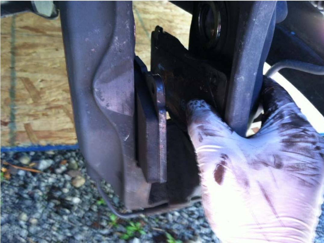
2. Remove the metal piece that is sitting on the back of the old pads. Use brake cleaner to clean the pins, retainer clip, and the metal backing plates. I also sprayed a towel and lightly cleaned off the piston area of the caliper.
