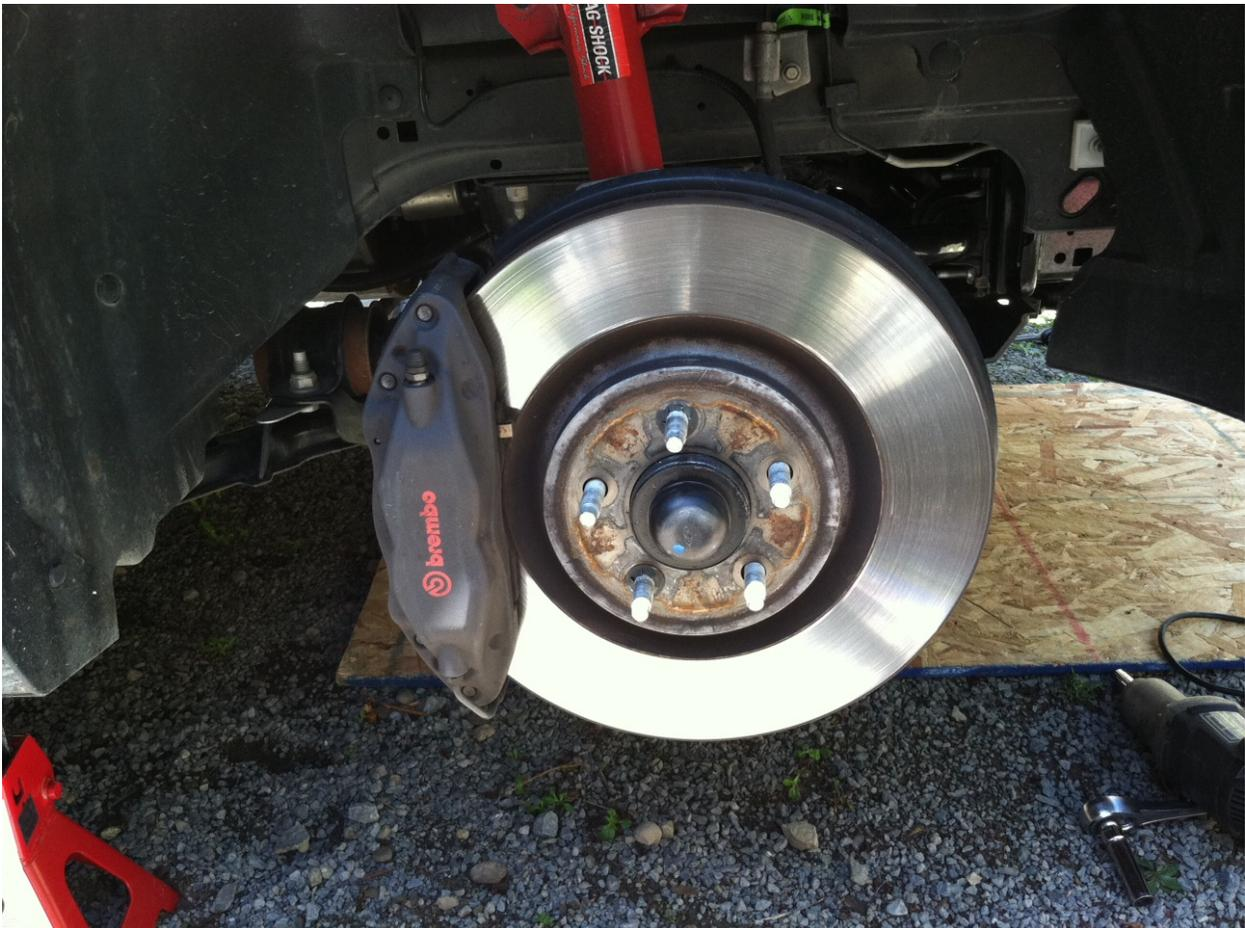
3. Use a hammer and center punch to begin to remove the pins holding the brake pads to the caliper. *Note: Take a look at the depth of the pin before removing so you will know when they are fully seated later.* Use CAUTION, the retainer clip that is held into place by the pins is under moderate pressure. Tap the pin until it is out far enough to grab with the channel locks. While removing the first pin the retainer clip will fly out, try deflecting the clip so it doesn't fly far.
