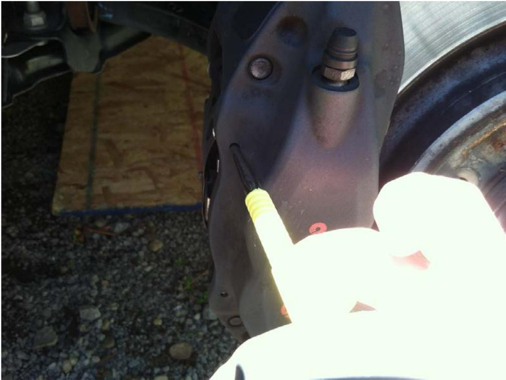
4. Once both pins and the retainer clip are removed you need to secure the caliper with wire to prevent brake line and caliper damage. I found it easiest to run the wire along the top of the rotor through the first part of caliper and then around the coil spring.
